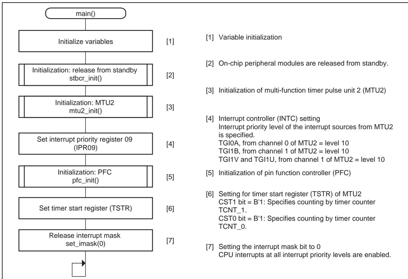
Figure 6 Processing by Function main
