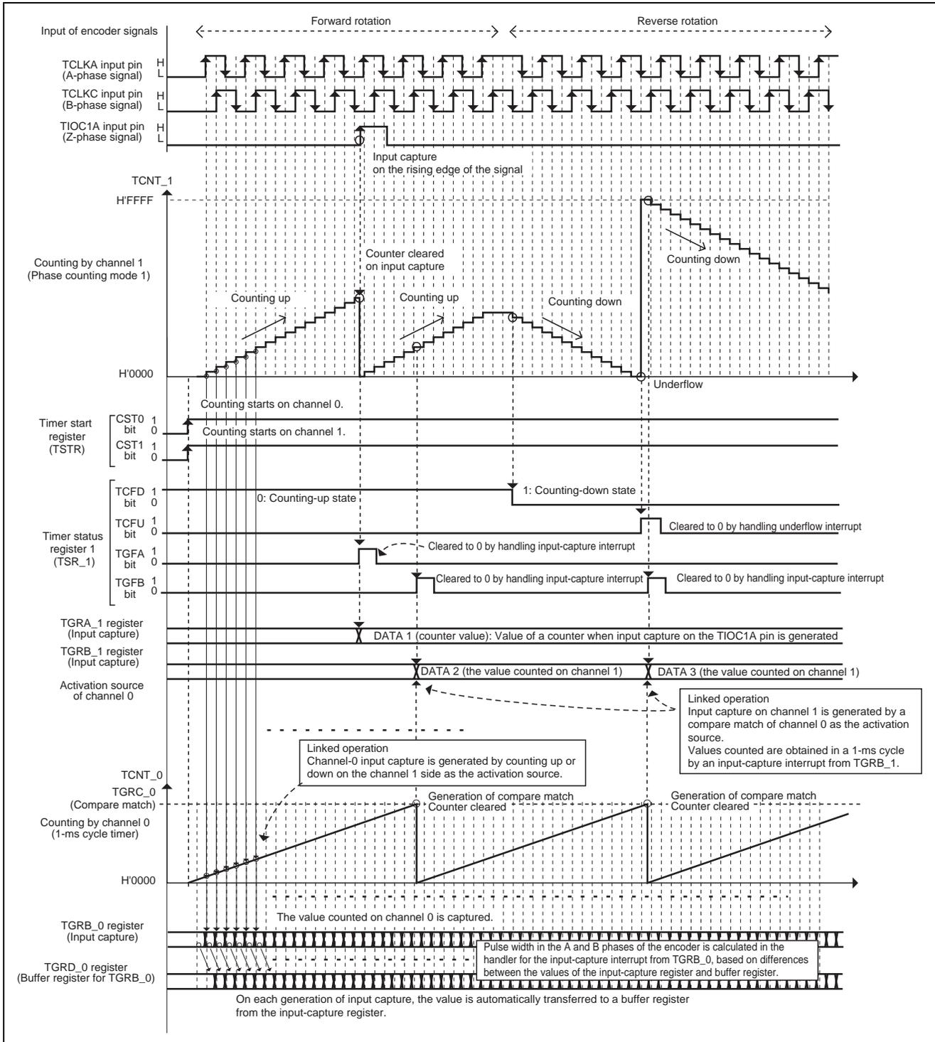
Figure 5 Operation Timing to Detect Signals of Two-Phase Encoder
