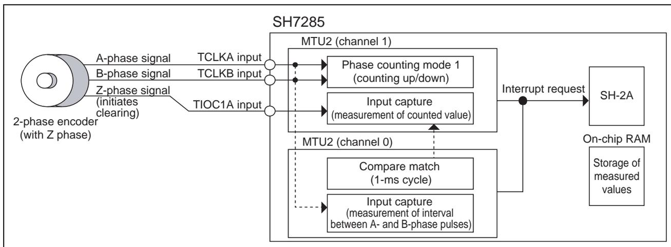
**Figure 1 Detection of Pulses from the Two-Phase Encoder (Phase Counting Mode 1)**
