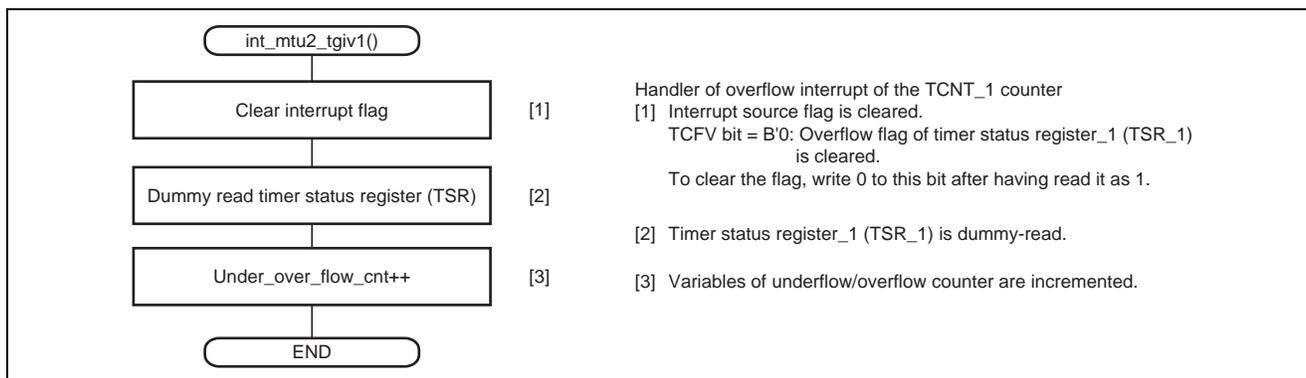
Figure 12 Handling of the Overflow Interrupt from Channel 1 of MTU2
