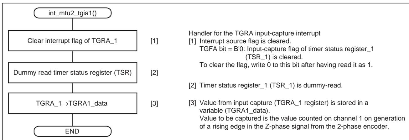
Figure 10 Handling of the Input Capture (TGRA\_1) Interrupt from Channel 1 of MTU2
