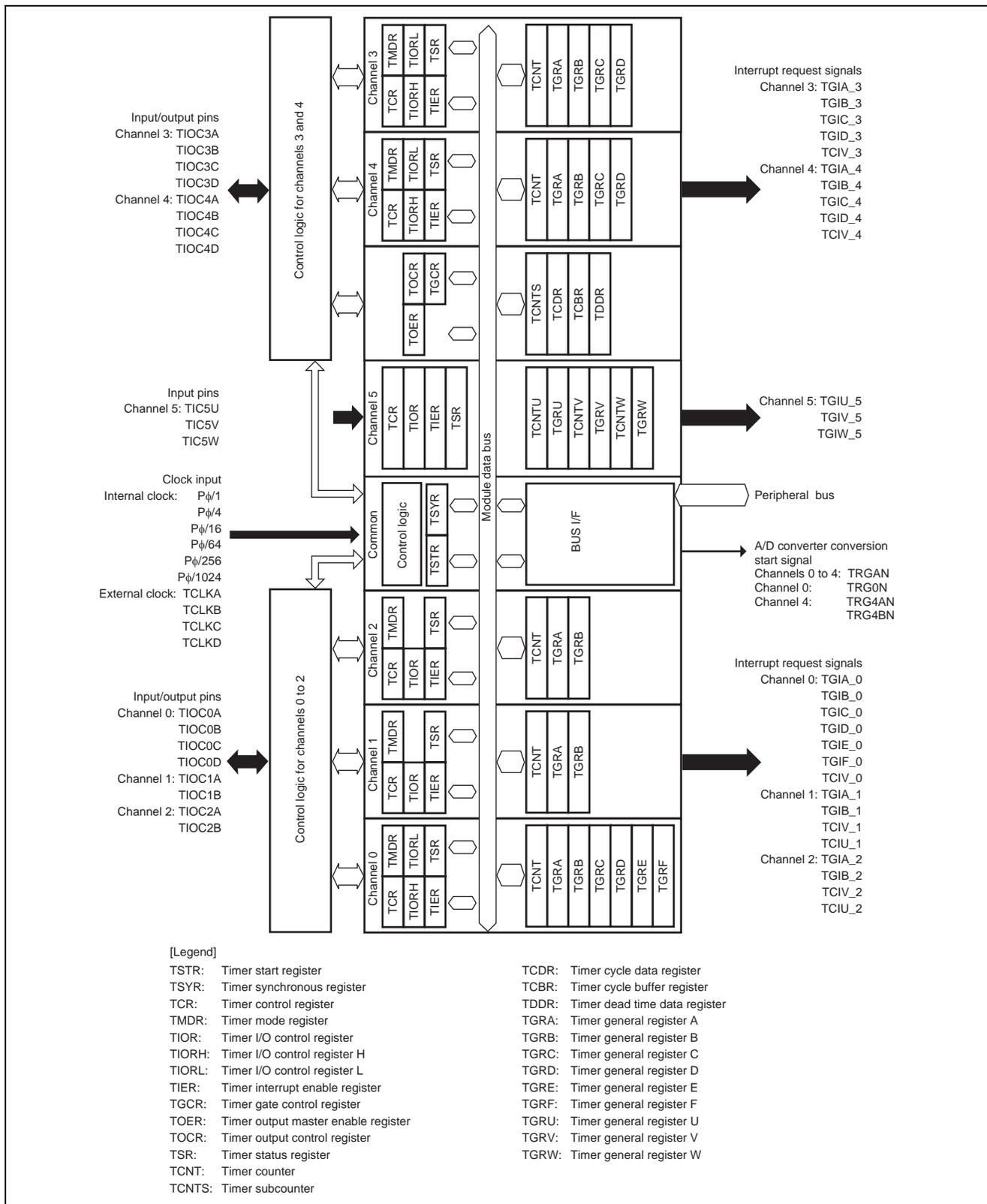
Figure 2 Block Diagram of MTU2
