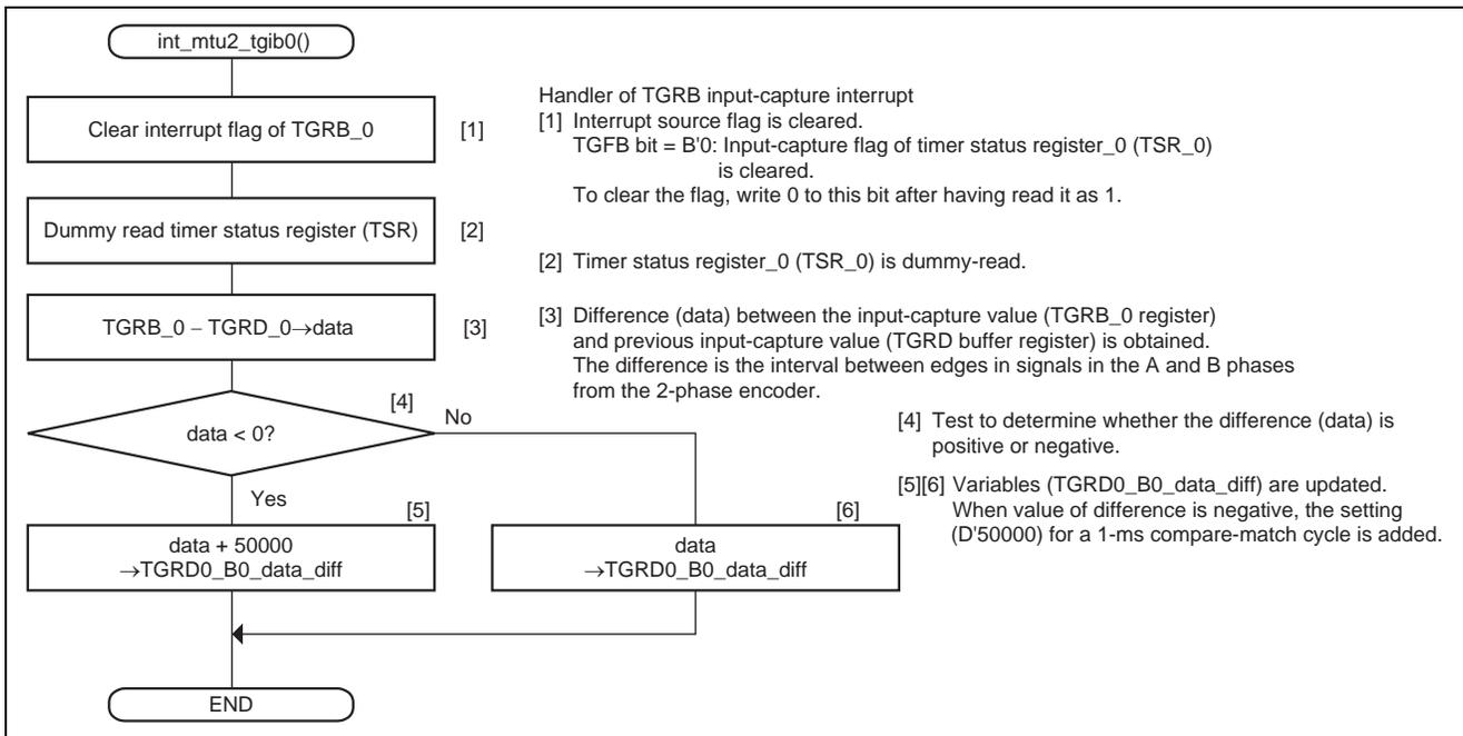
Figure 14 Handling of the Input Capture (TGRB\_0) Interrupt from Channel 1 of MTU2
