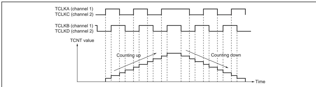
**Figure 3 Example of Operation in Phase Counting Mode 1 (Channels 1 and 2)**
