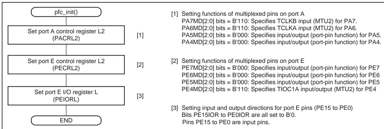
Figure 9 Flow for Setting PFC
