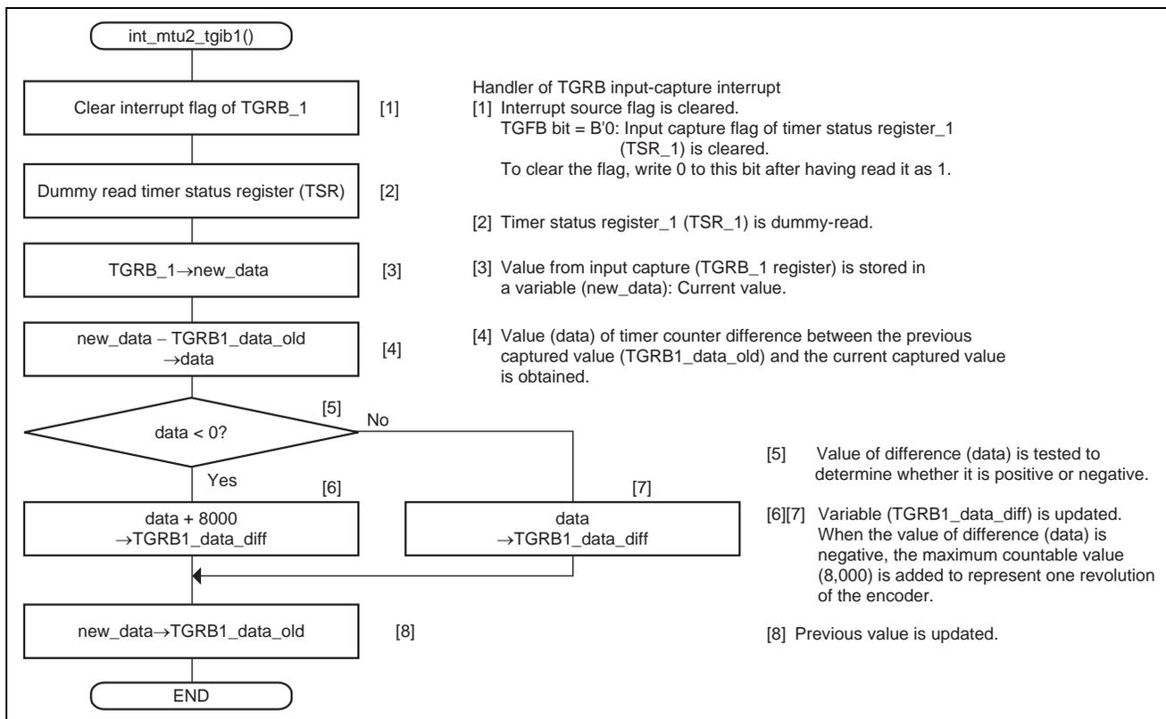
Figure 11 Handling of the Input Capture (TGRB\_1) Interrupt from Channel 1 of MTU2
