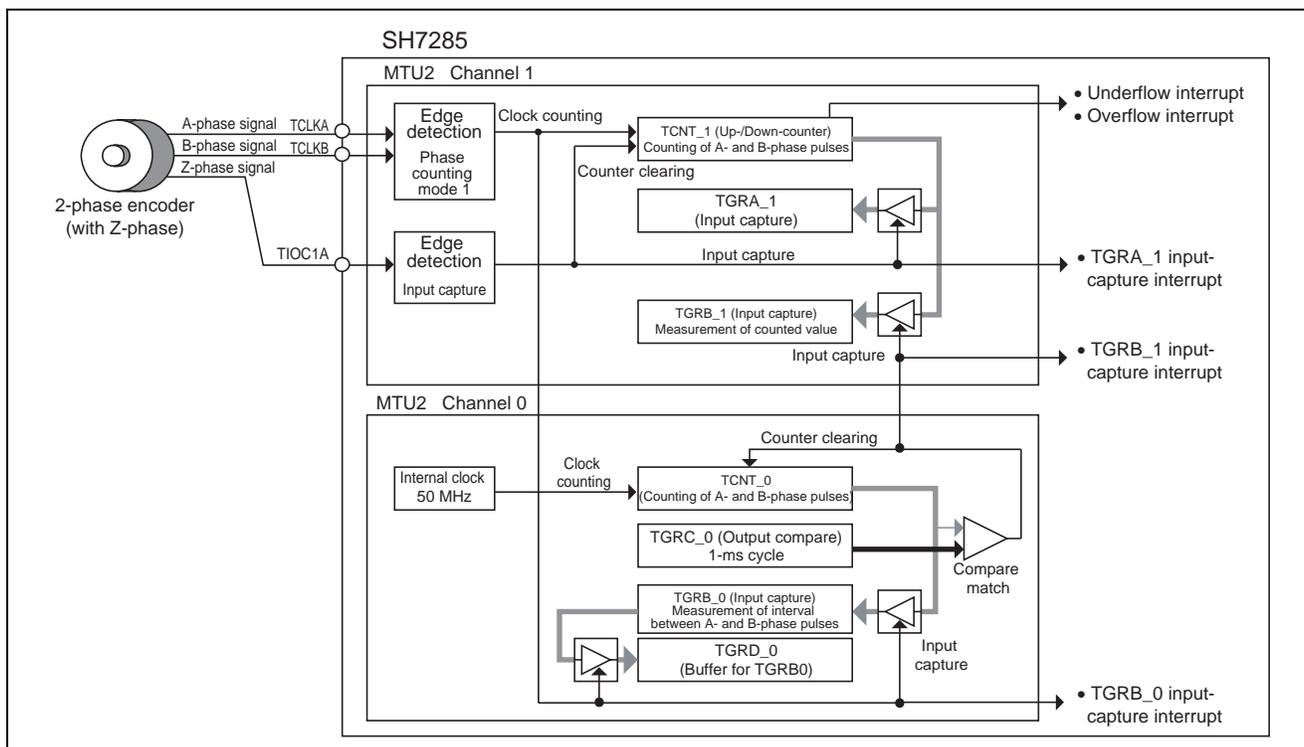
**Figure 4 Configuration of Channels 0 and 1 of MTU2**
