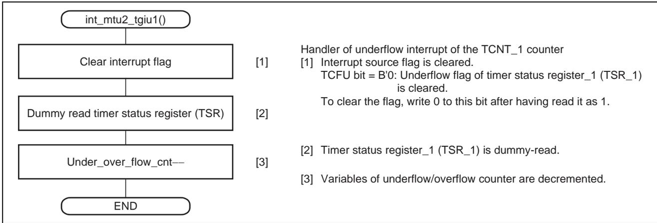
Figure 13 Handling of the Underflow Interrupt from Channel 1 of MTU2
