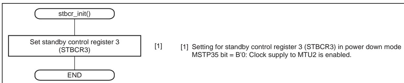
Figure 7 Setting for Release of the Module from Standby
