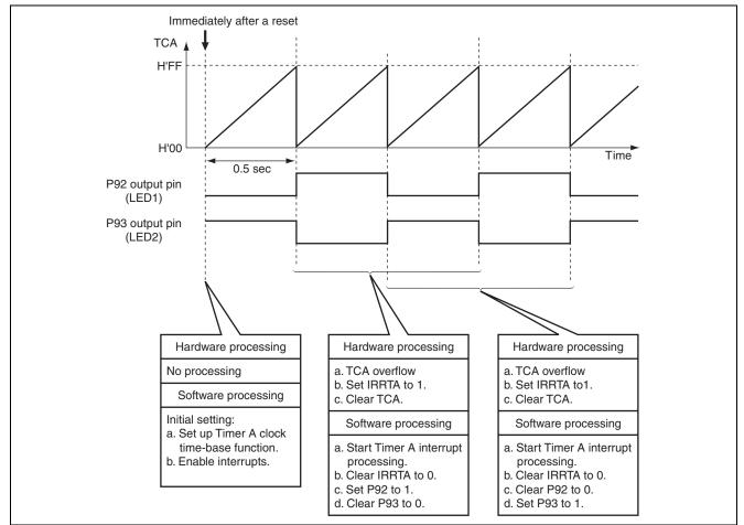
Figure 3.1 Operation Principle of Blinking of LEDs Connected to I/O Ports
