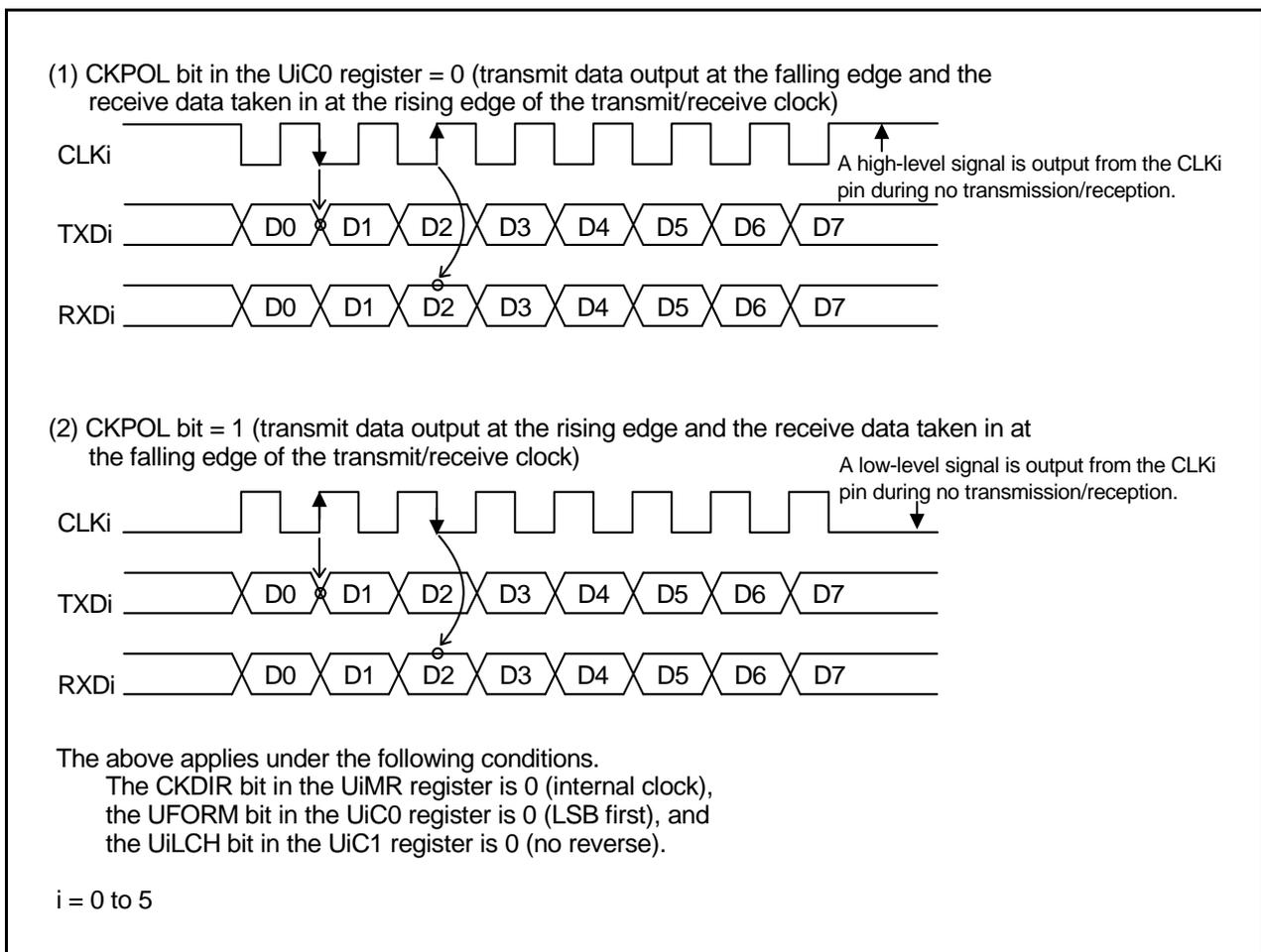
Figure 22.6 Transmit/Receive Clock Polarity
