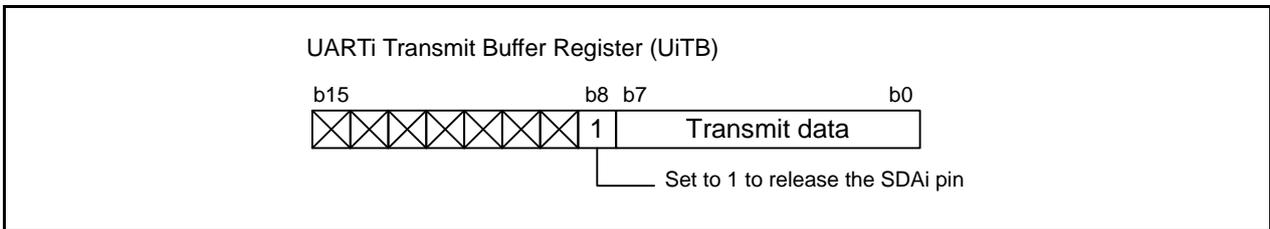
Figure 4.7 UiTB Register Setting (SDA Output)
