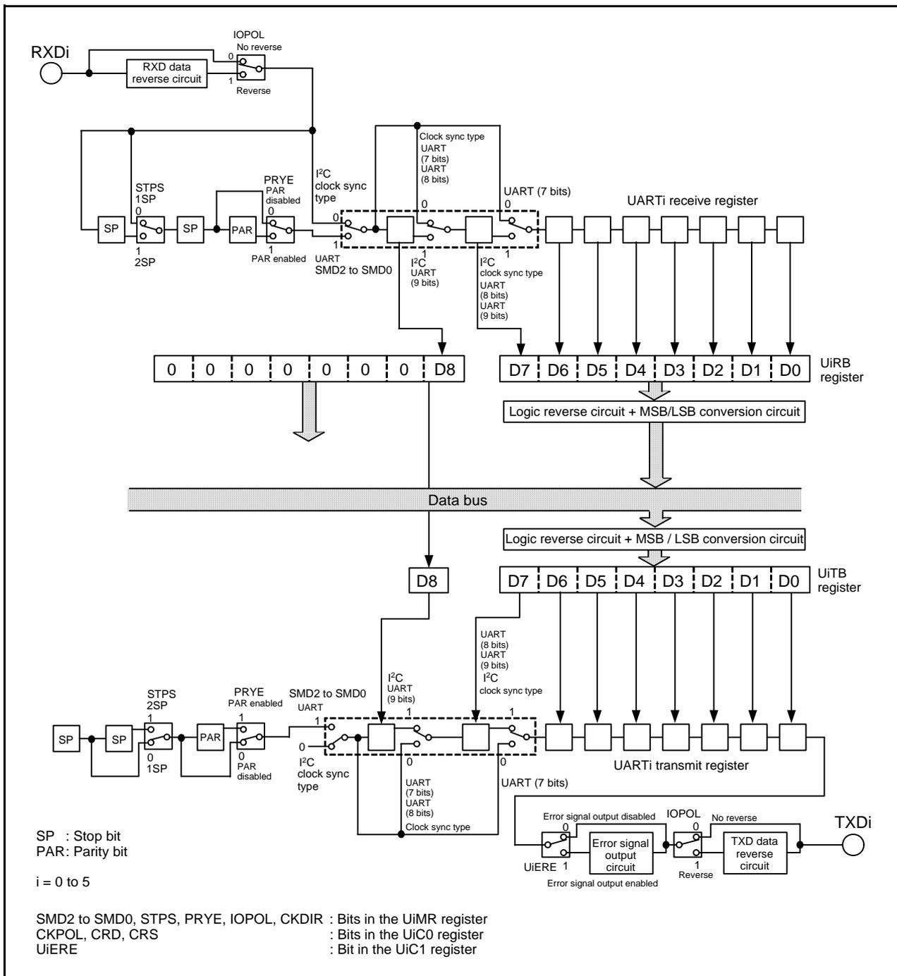
Figure 22.4 UARTi Transmit/Receive Unit Block Diagram
