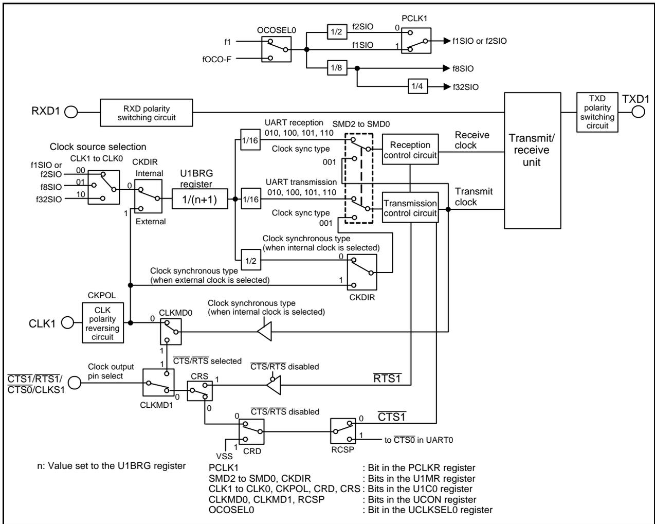
Figure 22.2 UART1 Block Diagram
