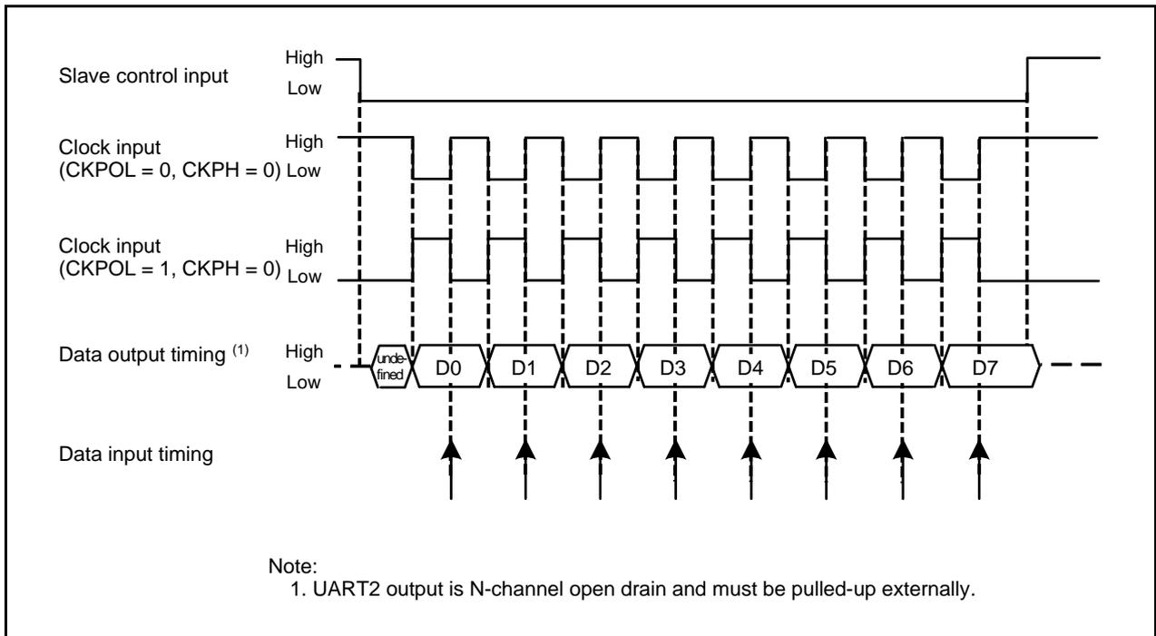
Figure 22.24 Transmission and Reception Timing (CKPH = 0) in Slave Mode (External Clock)
