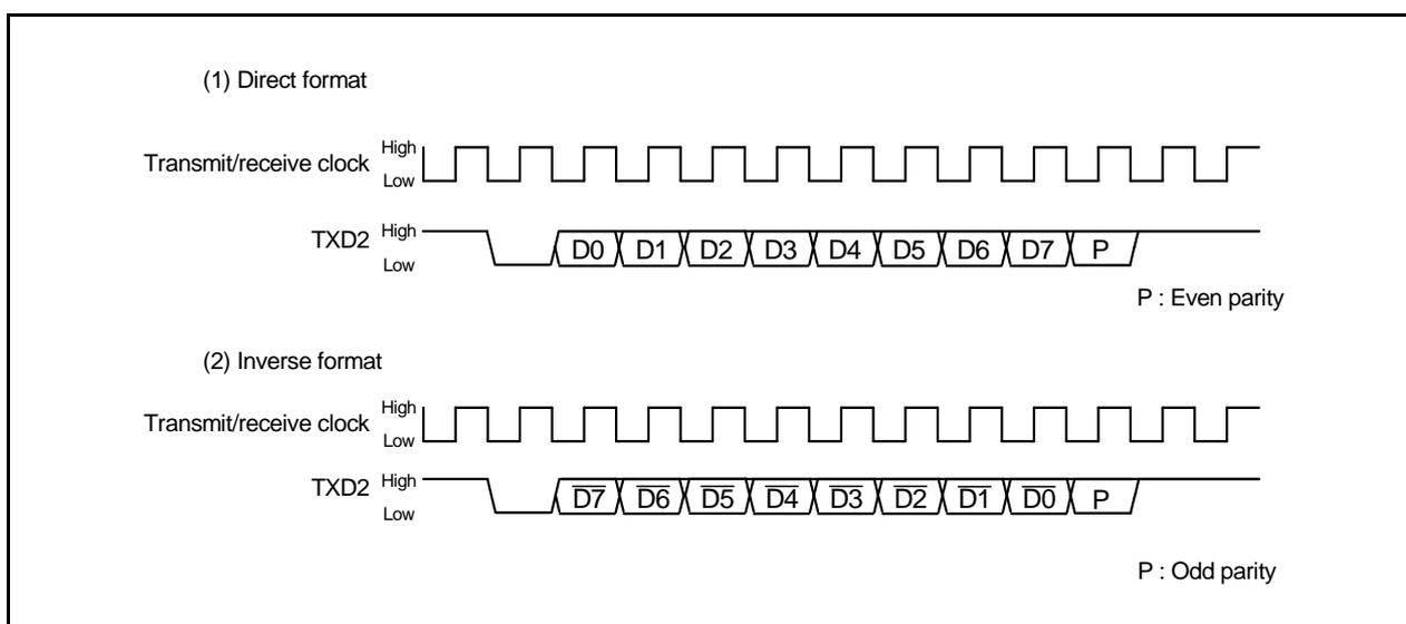
Figure 22.30 SIM Interface Format
