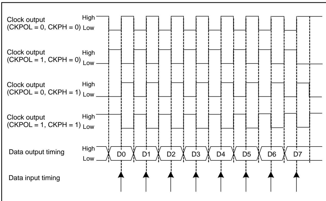
Figure 22.23 Transmission and Reception Timing in Master Mode (Internal Clock)
