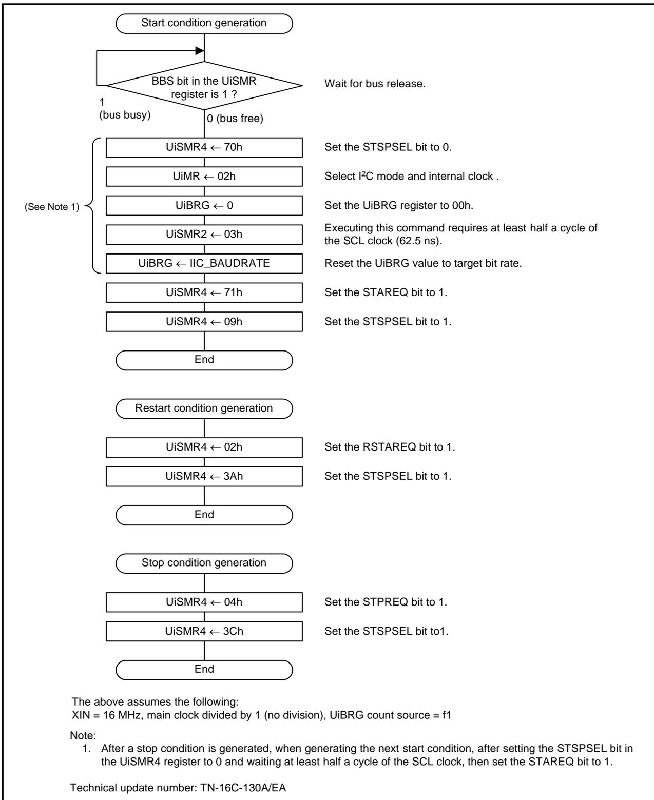
**Figure 4.3 Register Setting Procedures for Condition Generation**
