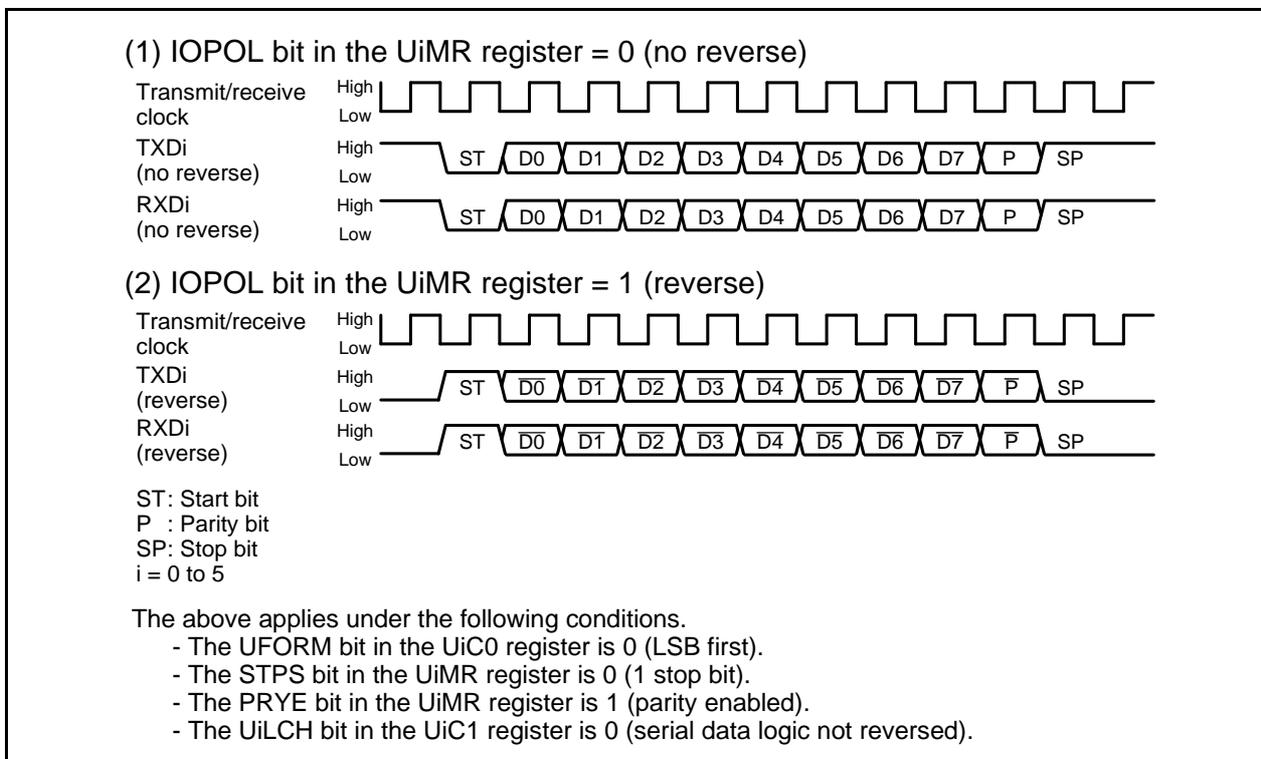
Figure 22.16 TXD and RXD I/O Polarity Reversal
