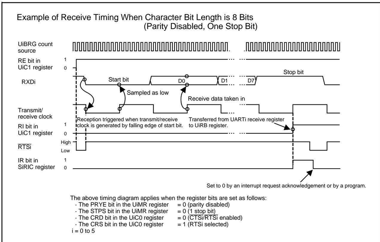
**Figure 22.13 Receive Timing in UART Mode**
