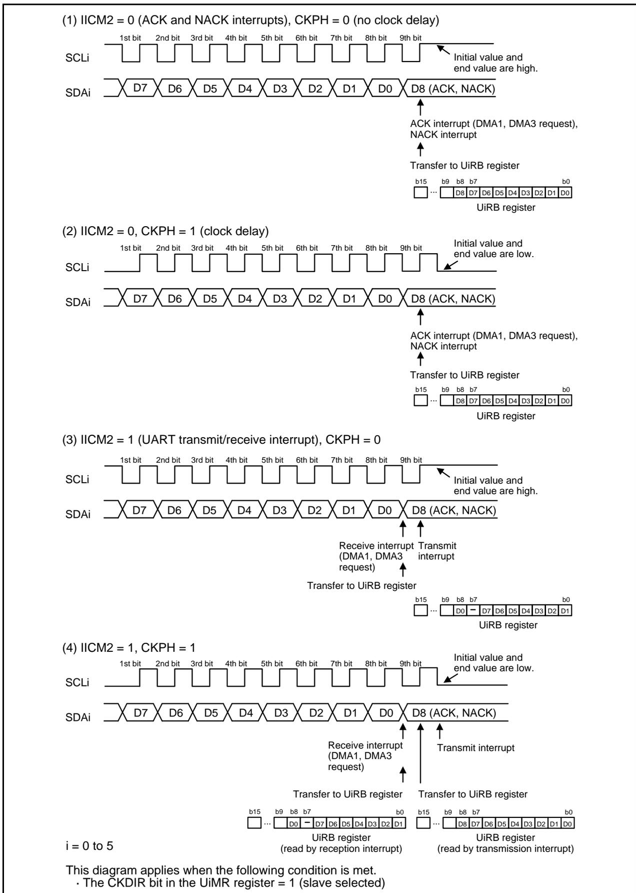
Figure 22.19 Transfer to UiRB Register and Interrupt Timing
