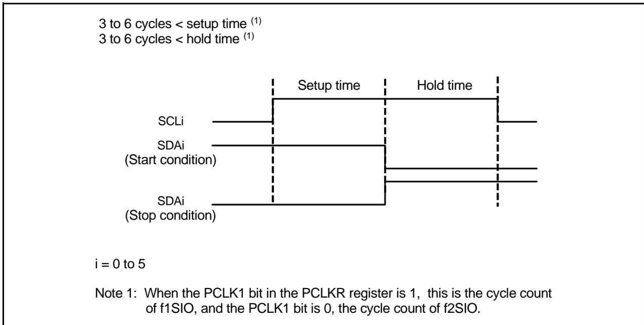
Figure 22.20 Detection of Start and Stop Conditions
