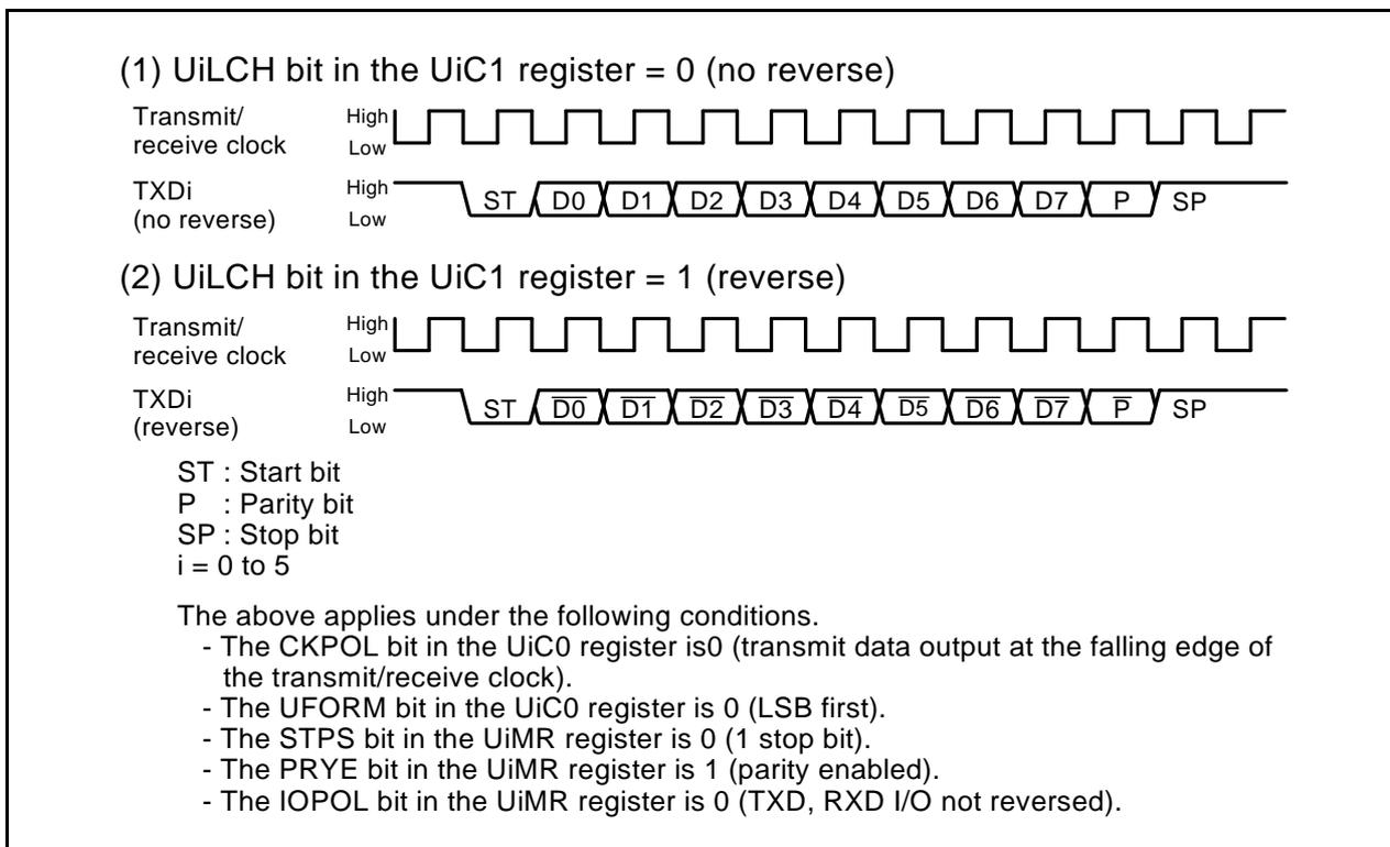
Figure 22.15 Serial Data Logic
