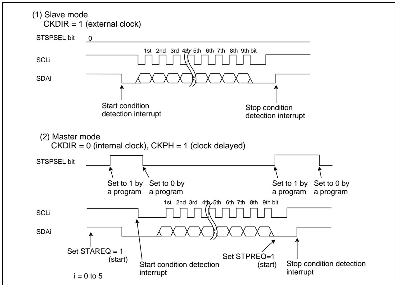
**Figure 22.21 STSPSEL Bit Functions**
