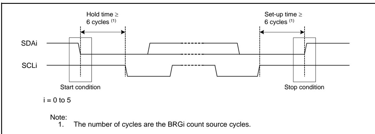
Figure 4.1 Detecting Start and Stop Conditions
