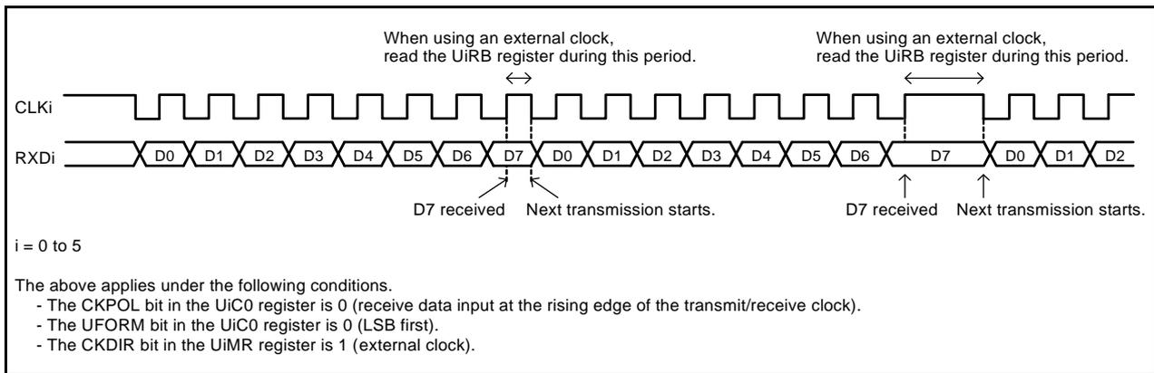
**Figure 22.8 Operation Example in Continuous Receive Mode**
