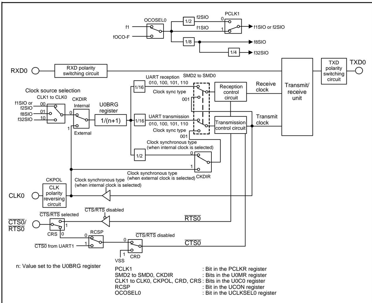
Figure 22.1 UART0 Block Diagram
