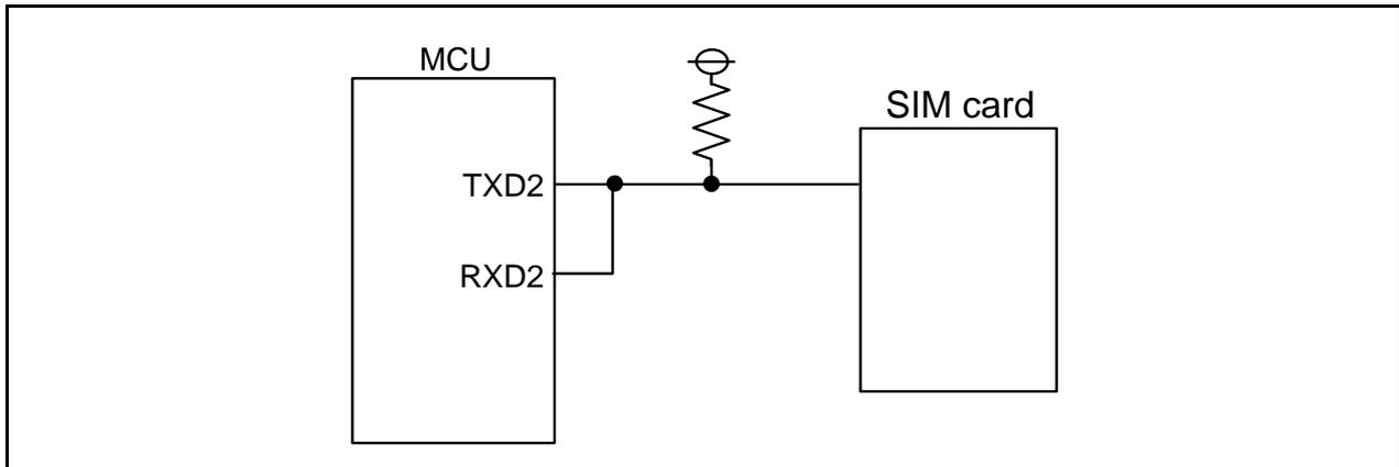
Figure 22.28 Example of SIM Interface Connection
