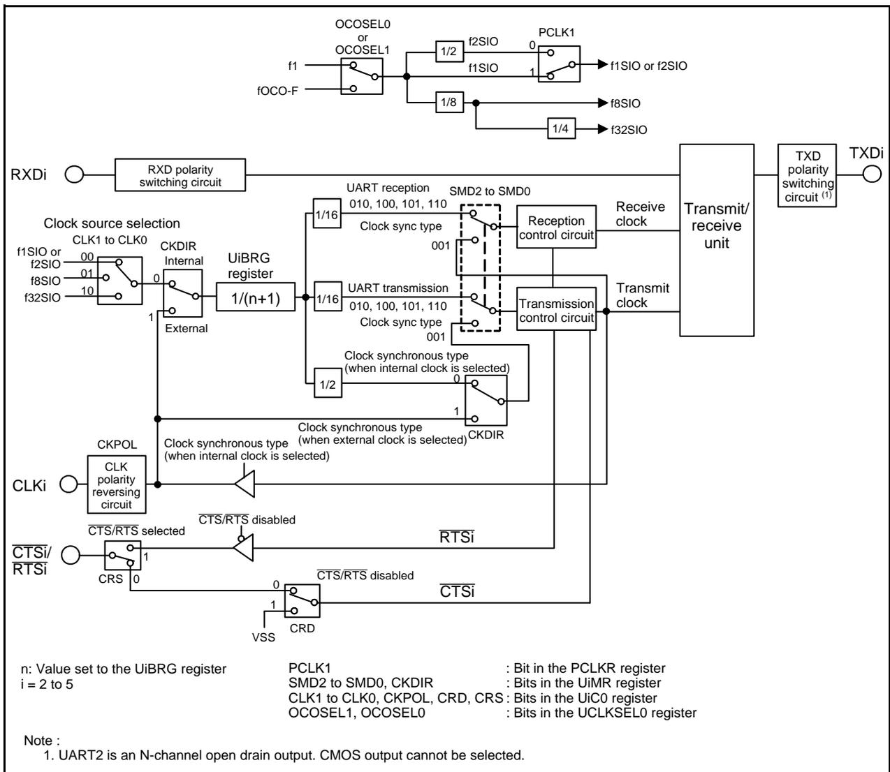
Figure 22.3 Block Diagram of UART2 to UART5
