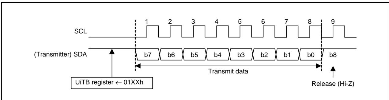
Figure 4.8 Byte Data Transmission
