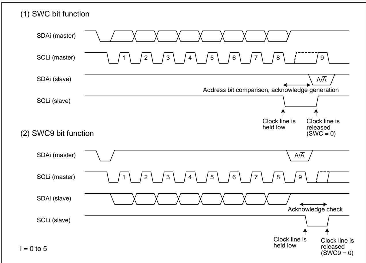
**Figure 4.4** Inserting Wait-states Using Bits SWC and SWC9
