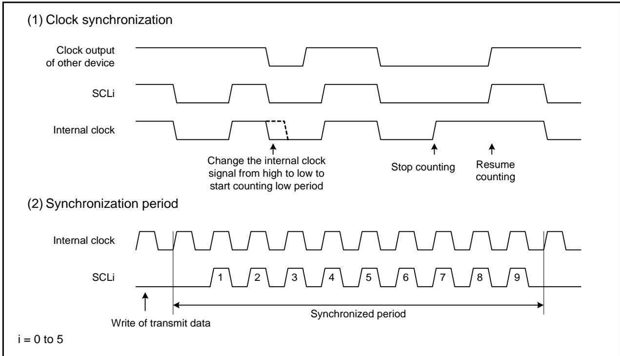
Figure 4.5 Clock Synchronization
