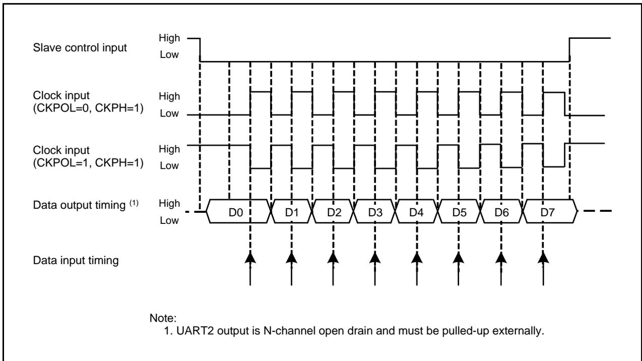
Figure 22.25 Transmission and Reception Timing (CKPH = 1) in Slave Mode (External Clock)
