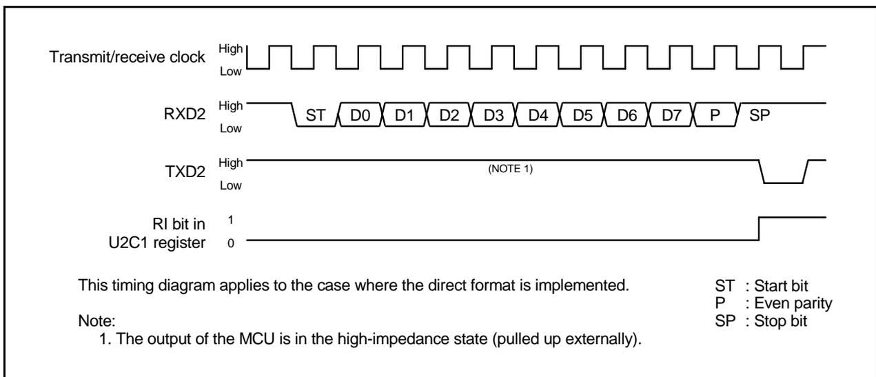
Figure 22.29 Parity Error Signal Output Timing
