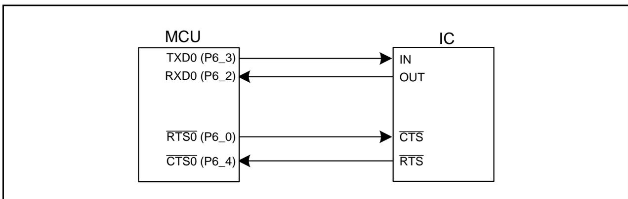
Figure 22.17  $\overline{\text{CTS}}/\overline{\text{RTS}}$  Separate Function
