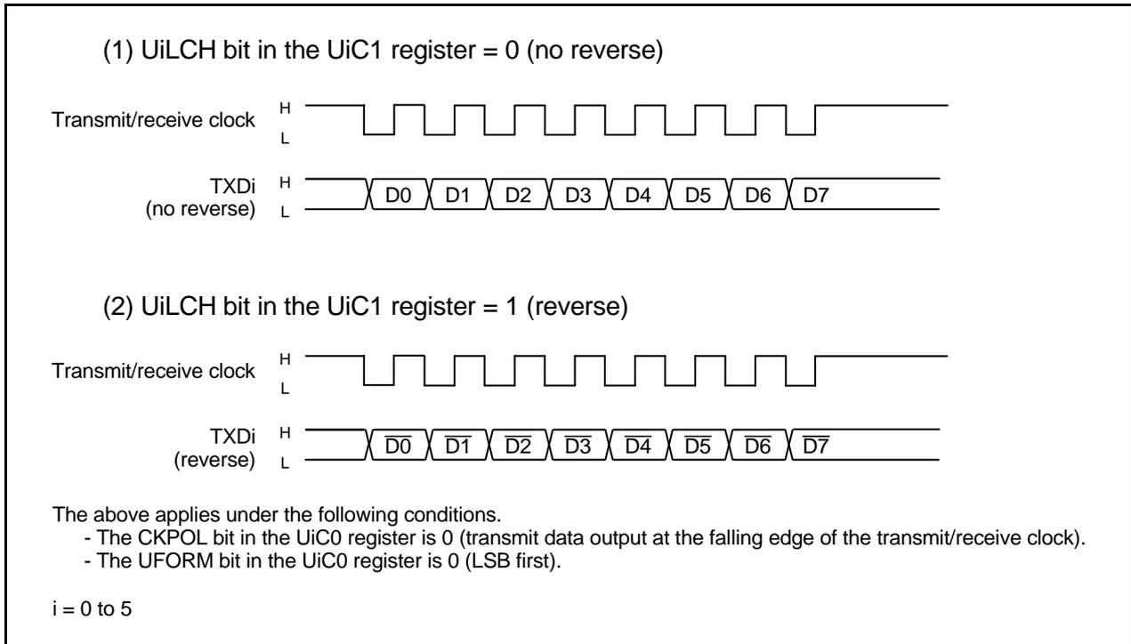
Figure 22.9 Serial Data Logic
