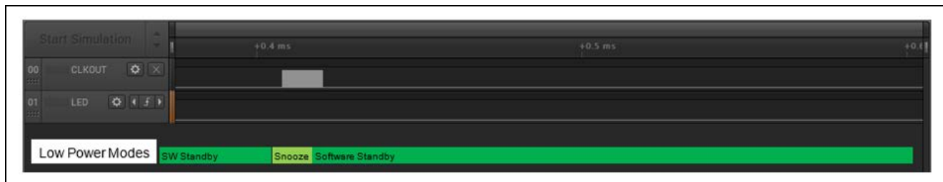
Figure 32. Example of Pin Output in Snooze Mode
