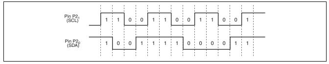
Figure 2.2 Pins P2<sub>1</sub> and P2<sub>0</sub> Timing Waveforms
