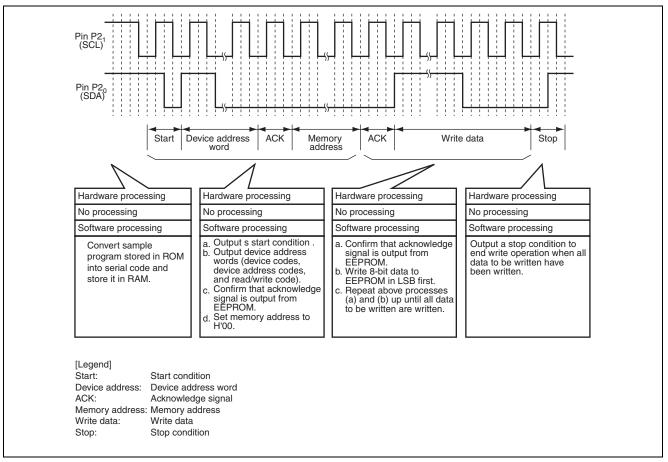
Figure 4.1 Principle of Operation during Writing to EEPROM
