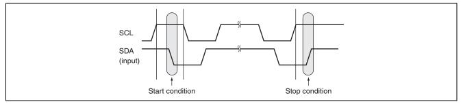
Figure 3.3 Start Condition/Stop Condition Set Timings
