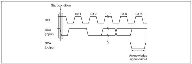
Figure 3.4 Acknowledge Signal Output Timings
