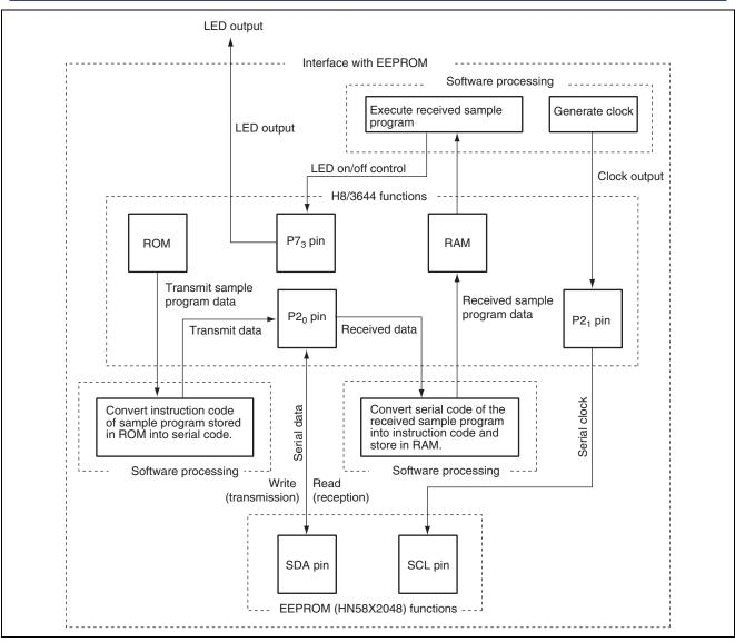
Figure 3.2 Block Diagram of Interface with EEPROM (HN58X2048)
