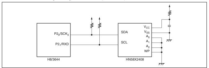
Figure 3.1 Connection between the H8/3644 and HN58X2408
