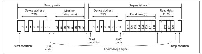
Figure 3.7 Sequential Read Operation
