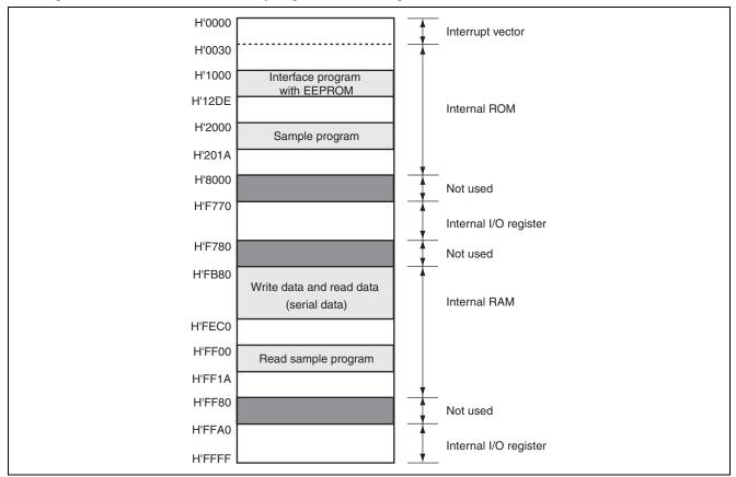
Figure 4.3 H8/3644 Memory Map used in this Sample Task
