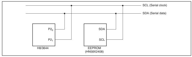
Figure 1.1 Connection between the H8/3644 and EEPROM
