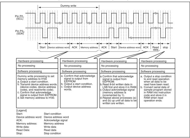
Figure 4.2 Principle of Operation during Reading from EEPROM
