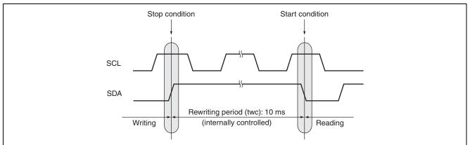
Figure 3.8 Rewrite Cycle Timings
