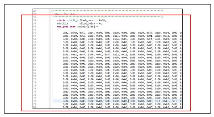
Figure 2 Assign Global Variable in "flashled.c"
