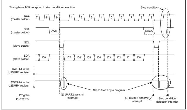
Figure 3.6 Slave Transmit Timing (2)
