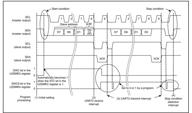
Figure 3.4 Slave Receive Timing
