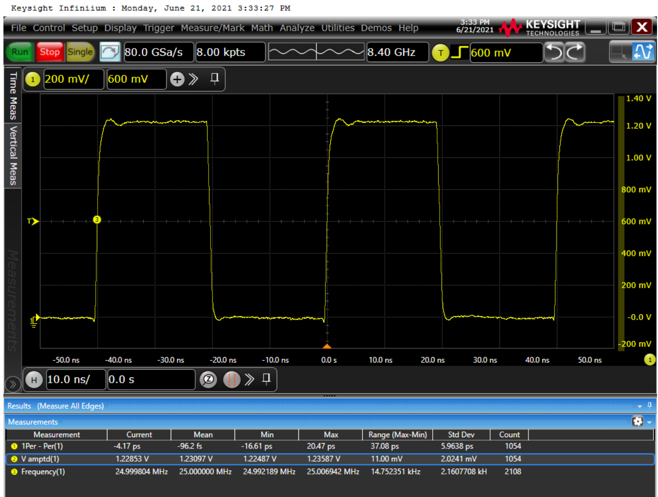
Figure 6. 1.8V LVCMOS 25MHz with 100Ω added at Receiver Side
