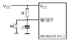
Figure 2.2 Reset Circuit II
