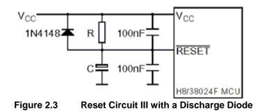
In Figure 2.3 above, the 1N4148 diode is used to rapidly discharge the C capacitor on power-down. This is very important, as a power-up reset pulse is needed after a short power-down (less than the time given by the RC constant) or after a power spike. The two 100nF capacitors allow the reset pin level to follow the voltage variations that appear on either VCC or VSS.
