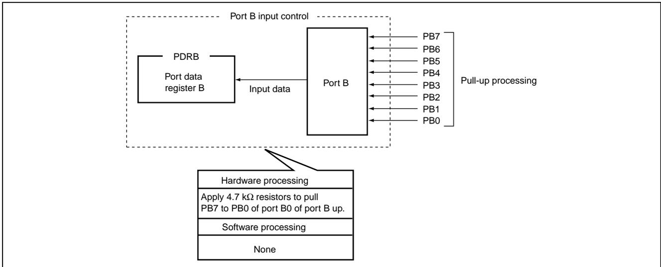
Figure 3.3 Processing for Open-Circuit Pins of Input Ports (e.g. Port B)
