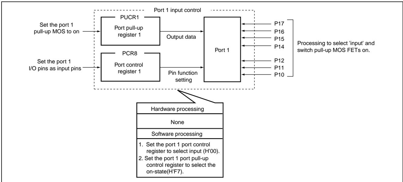
Figure 3.1 Processing for Open-Circuit Pins of Ports with Pull-Up MOSFETs (e.g. Port 1)
