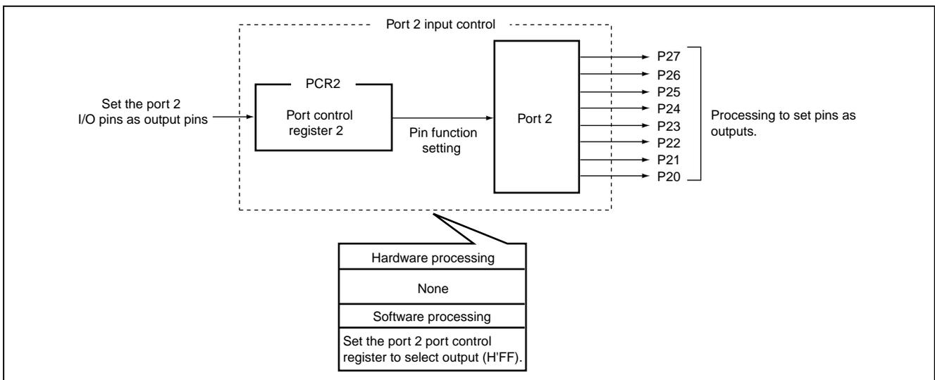
Figure 3.2 Processing for Open-Circuit Pins of General I/O Ports (e.g. Port 2)
