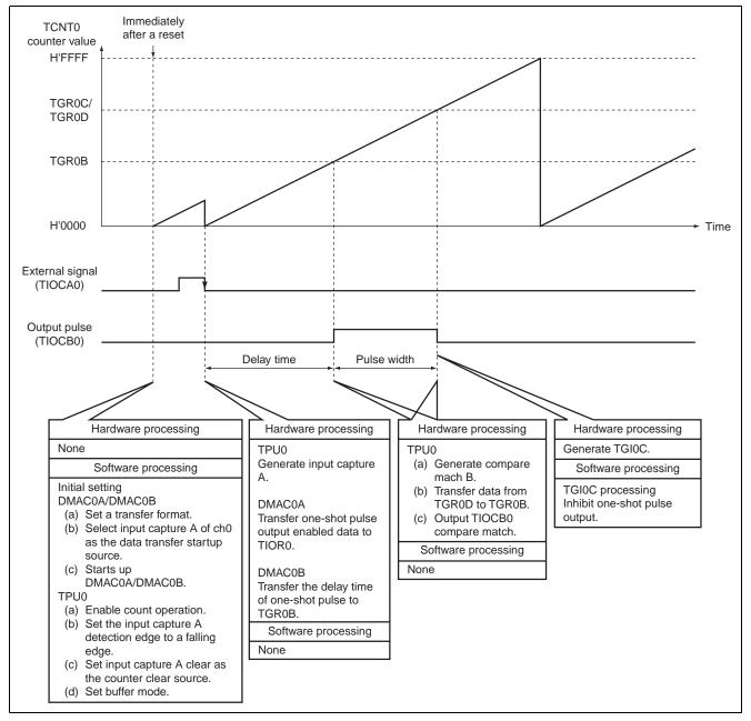
Figure 3 Principles of Operations Used of One-Shot Pulse Output
