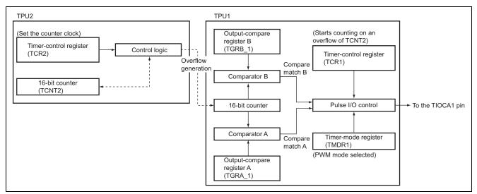
Figure 2 Block Diagram of Long-Cycle Pulse Output
