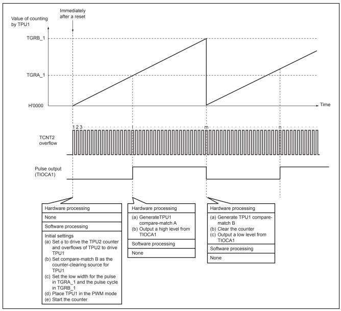
Figure 3 Output of the Long-Cycle Pulse
