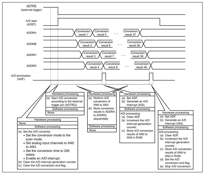
Figure 3 Principles of Operations Used for A/D Conversion in the Scan Mode
