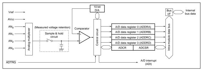
Figure 2 A/D Converter Block Diagram
