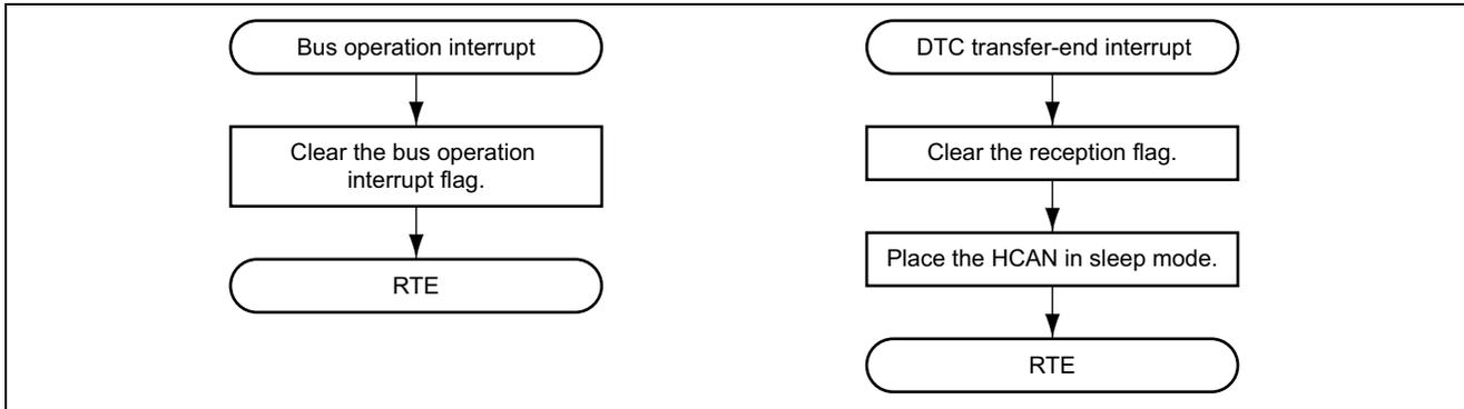
Figure 3 Flowchart of Interrupt Routines for the Receiver
