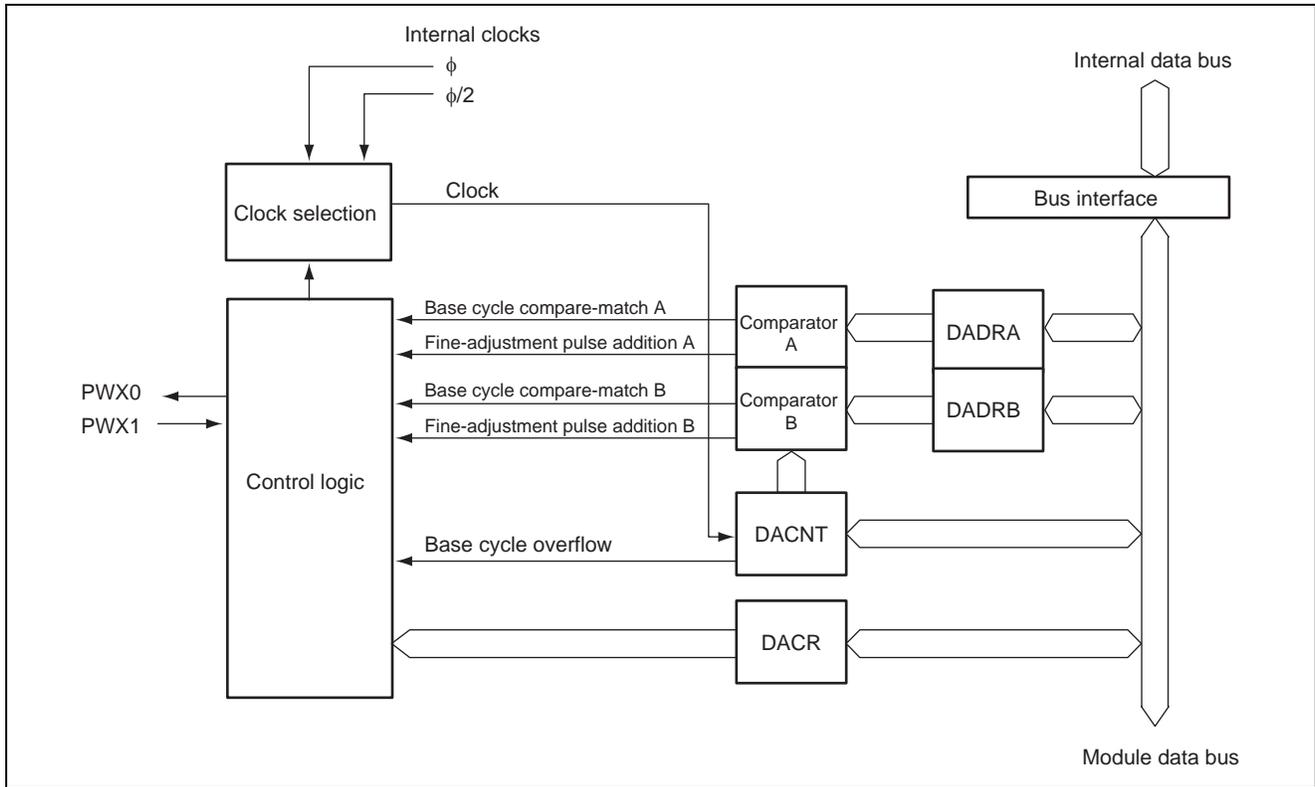
Figure 2 Block Diagram of 14-bit PWM Function
