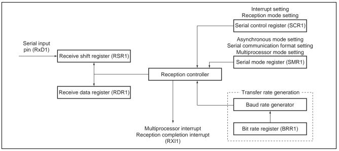
Figure 3 Block Diagram of Receiving Station SCI
