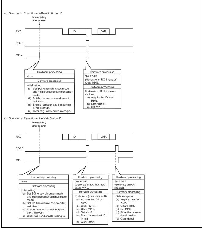
Figure 5 Principles of Operations Used of Multiprocessor Communication (Receiving Station)
