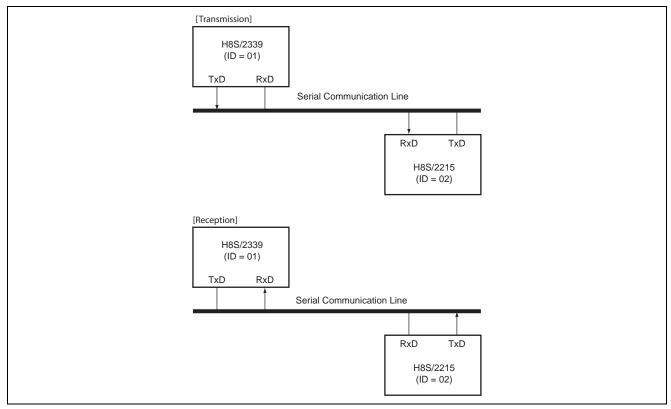
Figure 1 Block Diagram of Asynchronous SCI Using Multiprocessor Function
