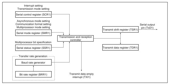
Figure 2 Block Diagram of Transmitting Station SCI
