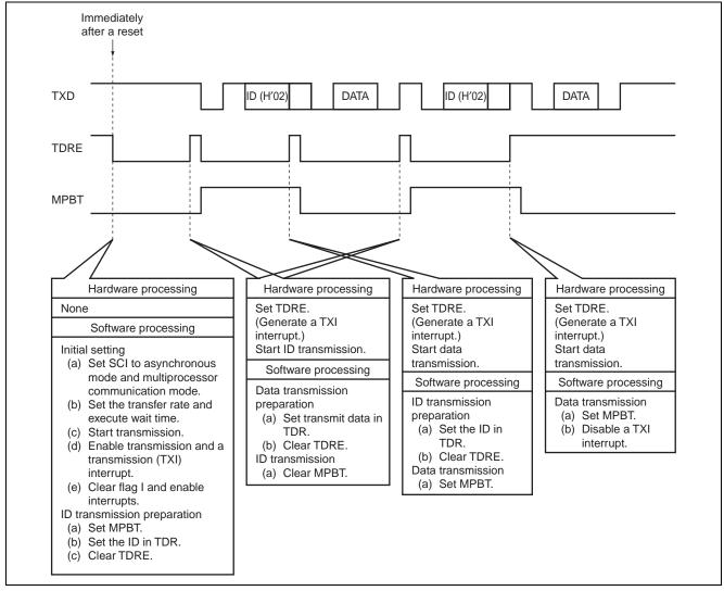
Figure 4 Principles of Operations Used for Multiprocessor Communication (Transmitting Station)
