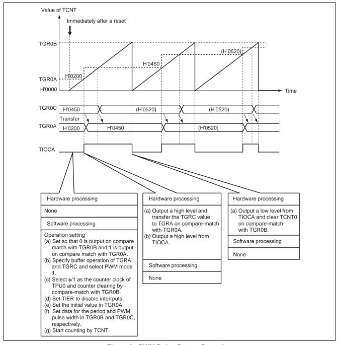
Figure 3 PWM Pulse Output Operation
