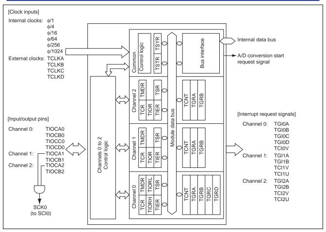
Figure 2 Block Diagram of TPU
