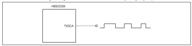
Figure 1 Example of PWM Waveform Output by TPU Buffer Operation
