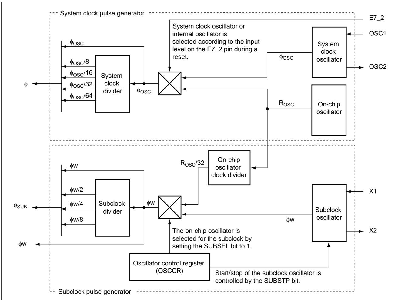
Figure 2 Block Diagram of Clock Pulse Generators
