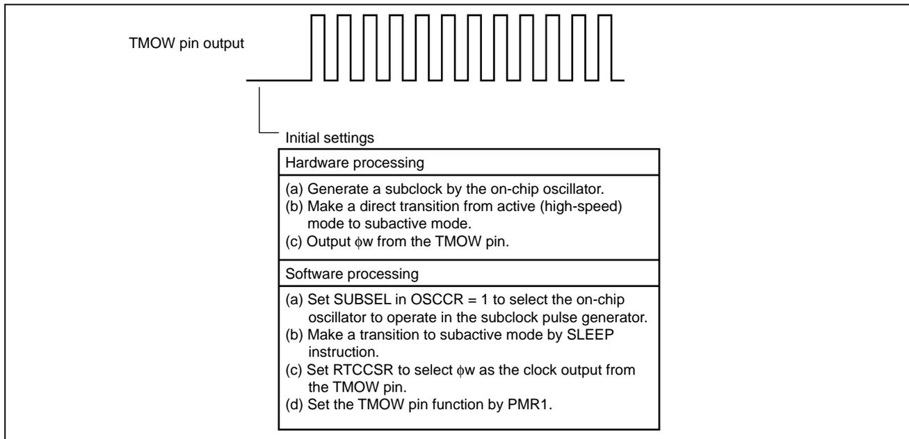
**Figure 4 Subclock Operation by On-chip Oscillator**
