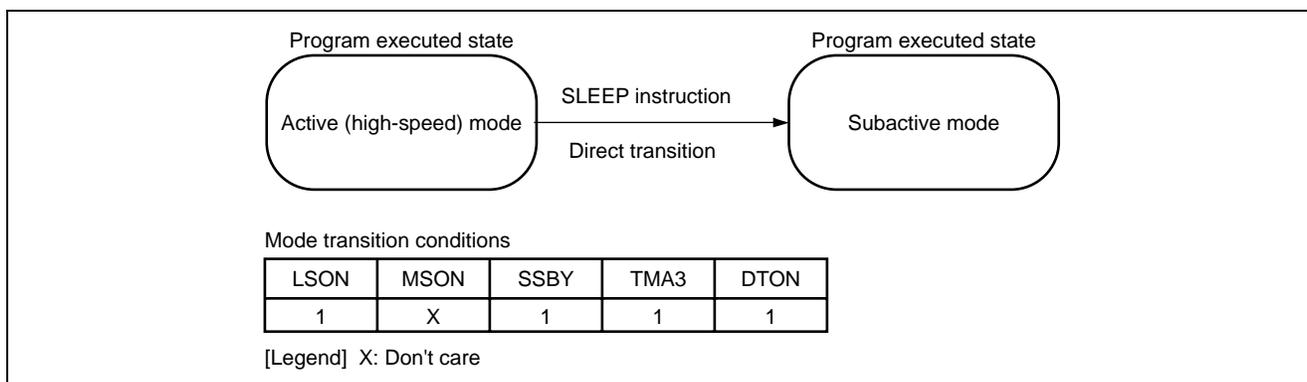
**Figure 3 Direct Transition from Active (High-Speed) Mode to Subactive Mode**
