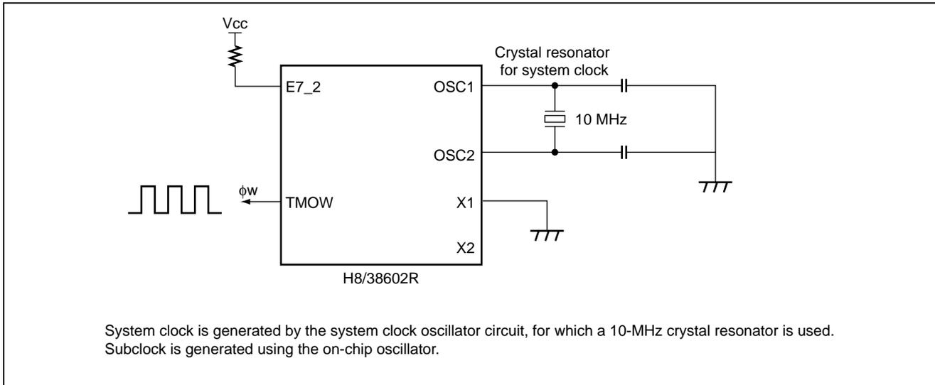
Figure 1 Subclock Operation Using On-chip Oscillator
