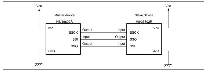
Figure 1 Connections in Clocked Synchronous Communication Mode of SSU
