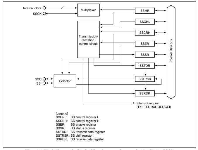
Figure 2 Block Diagram in Clocked Synchronous Communication Mode of SSU
