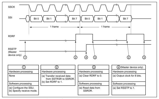
Figure 4 Operation Timing in Receive Mode
