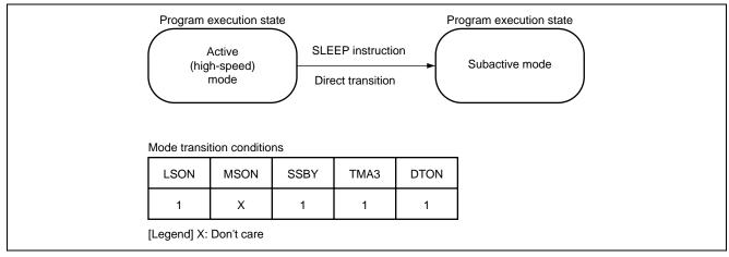
Figure 3 Direct Transition from Active (High-Speed) Mode to Subactive Mode
