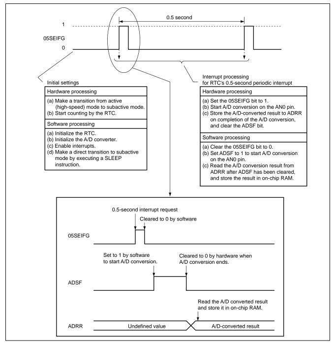
Figure 4 Principles of Operation
