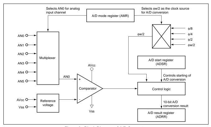
Figure 2 Block Diagram of A/D Converter
