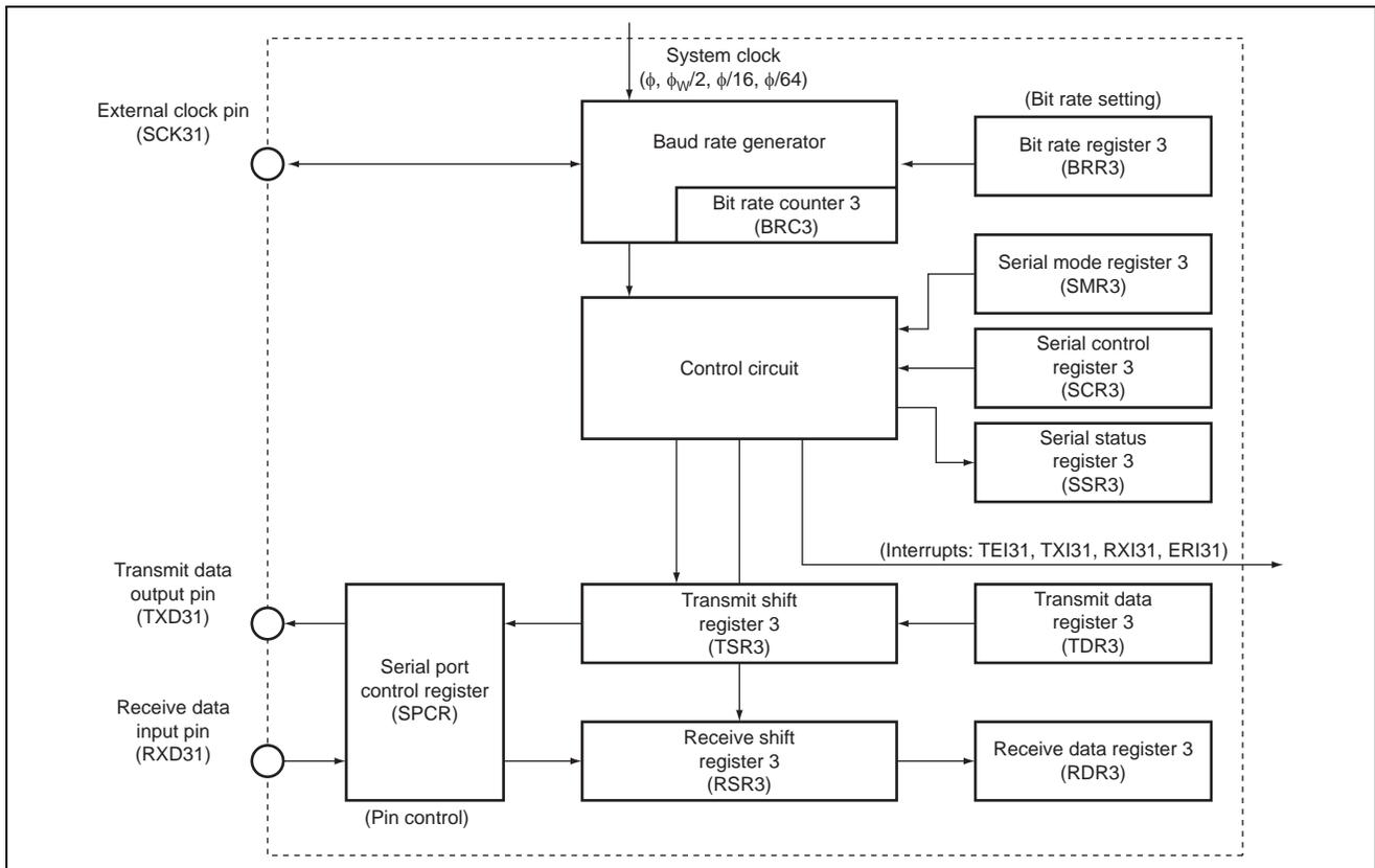
Figure 3 Block Diagram of SCI3
