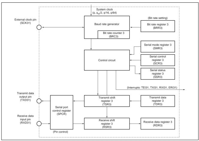
Figure 2 Block Diagram of SCI3
