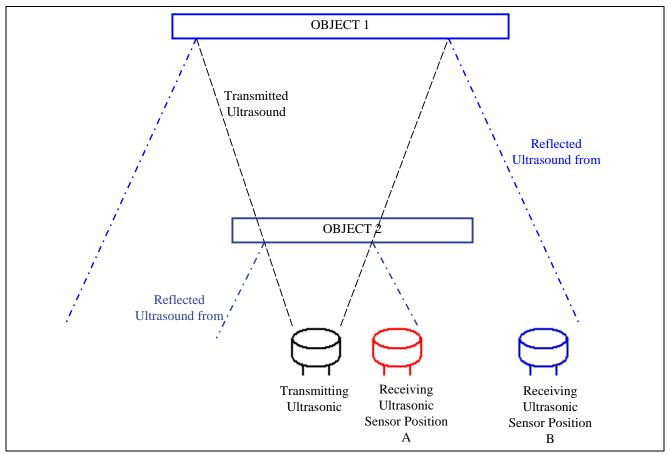
Figure 9 Illustration of Difference Between Distances of Sensors
