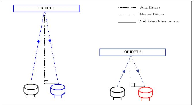
Figure 10 Illustration of Actual Distance Measured
