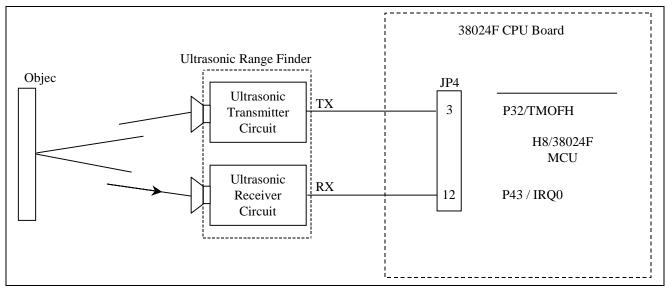
The H8/38024F CPU board is connected to the Ultrasonic Range Finder circuit as shown in figure 6:
