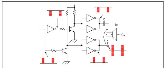
Figure 3 Transmitter Circuit
