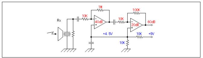
Figure 4 Signal Amplification Circuit
