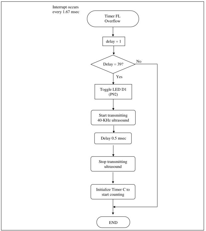
Figure 10 Timer FL Overflow Interrupt Service Routine
