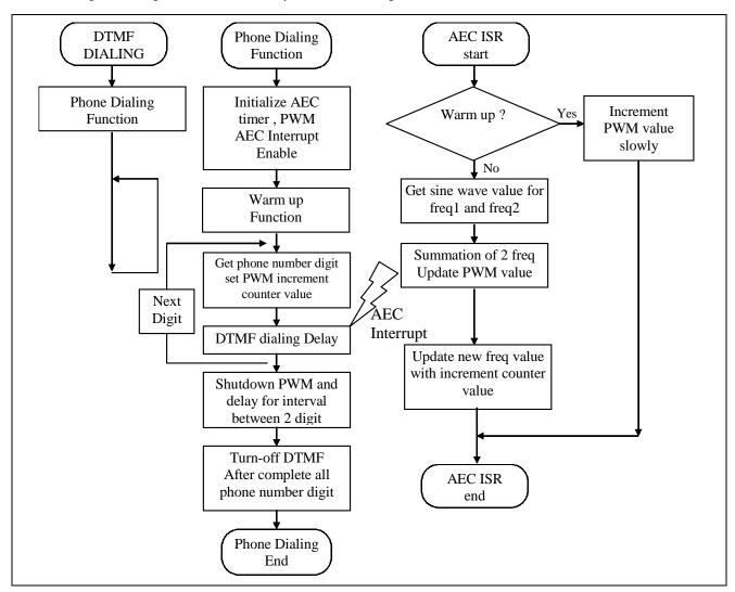
Figure 10 Flow Chart for DTMF\_dialing.c
