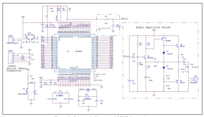
Figure 7 Schematic Diagram of DTMF Generation
