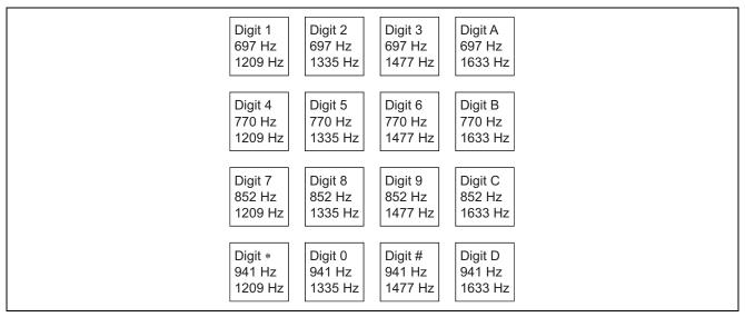
Figure 1 Keypad Digits and Frequencies of Tone Pairs
