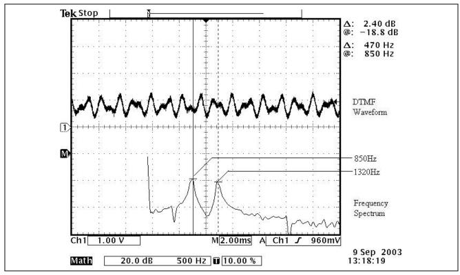
Figure 9 DTMF Waveform and Frequency Spectrum for Digit '8' (Peak Frequencies)
