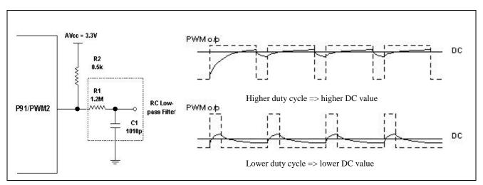
Figure 3 PWM to D/A Converter Example
