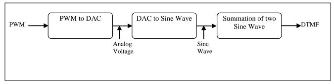
Figure 2 Overview of DTMF Signal Generation Process
