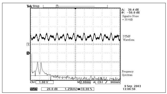
Figure 8 DTMF Waveform and Frequency Spectrum for Digit '8' (SNR)
