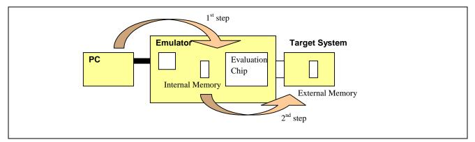
If the downloaded area is within the emulator (internal memory), the speed will be fast. However if the downloaded area is at external target area, it will need to transfer the data from the PC to the emulator (internal), and through the evaluation chip, transfer the data out to the external target area. This mechanism will be further slowed down if the user configure the evaluation chip to a slow operating frequency.
