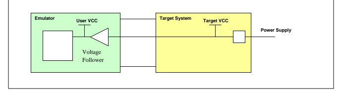
From the above diagram, Hardware developers can rest assured that the emulators will not draw current from the target. The emulator will generate an internal voltage (User Vcc) for internal operation, which is based on a target system supply (Target Vcc). When current measurement is made on the target, developers will have to take into the account that the emulating MCU is not consuming the target power.
