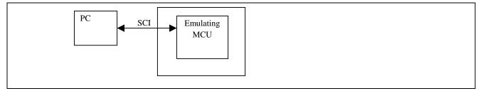
Another implementation is to directly use the emulating MCU serial port's interrupt to perform the communication. Thus user program shall not disable the interrupt, if otherwise the PC will not be able to communicate with the MCU.
