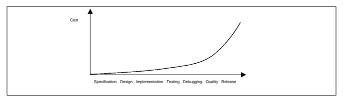
2. More effort is required during integration (testing and debugging) than implementation stage.
