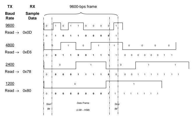
The transmitter's serial data stream, which is based on the different baud rate, will be fed into the 9600-bps receiver. Data will be sampled at this rate. The first data bit will be the LSB (least significant bit).
