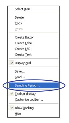
Clicking on the [Sampling Period...] item brings up the [Update View] dialog box. The interval value is specifiable to adjust the interval for updating of the [GUI I/O] window within the range from 10 ms to 10 s.
