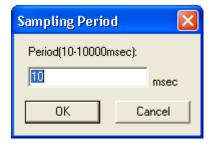
When an address value that has been specified for an item of the GUI I/O function is updated by the user program, the state of the item will be reflected in the [GUI I/O] pane each time the interval for updating of the display specified here elapses.
