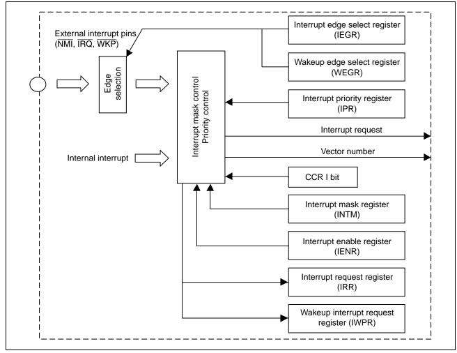
Figure 2 Block Diagram of Interrupt Controller
