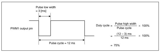
Figure 1 Duty Pulse Output Using Event Counter PWM Output Function of AEC
