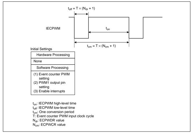
Figure 3 Principles of Operation
