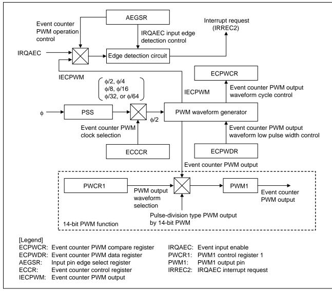
Figure 2 Block Diagram of AEC Event Counter PWM Output Function
