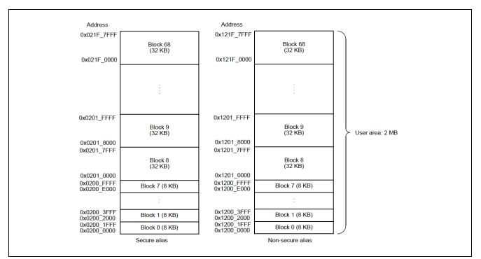
Figure 23. RA8 Map of the Code Flash Memory in Linear Mode
