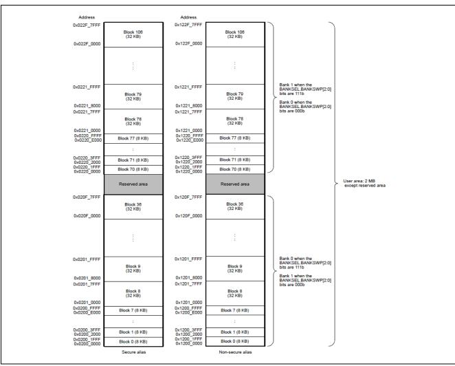
Figure 24. RA8 Map of the Code Flash Memory in Dual Mode
