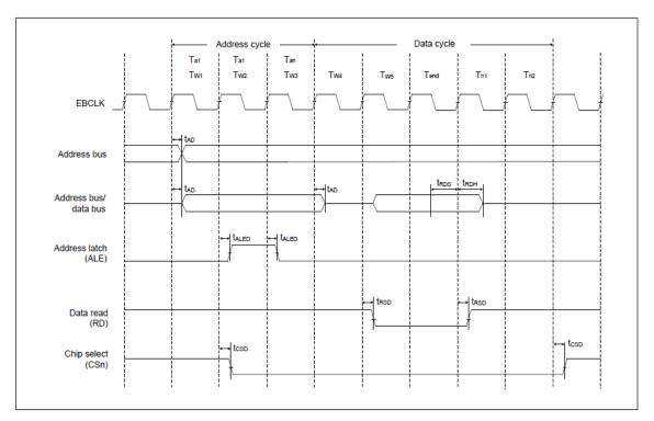
Figure 39. Address/data Multiplexed Bus Read Access Timing
