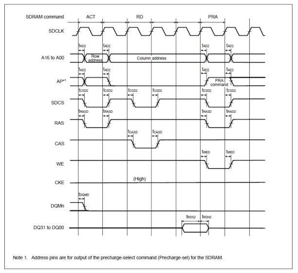
Figure 40. SDRAM Single Read Timing
