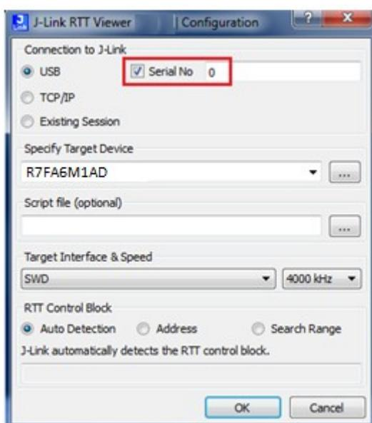
4. For parts other than Cortex-M33, click **OK**. For MCUs based on Cortex M33 Core, refer to the Appendix.
