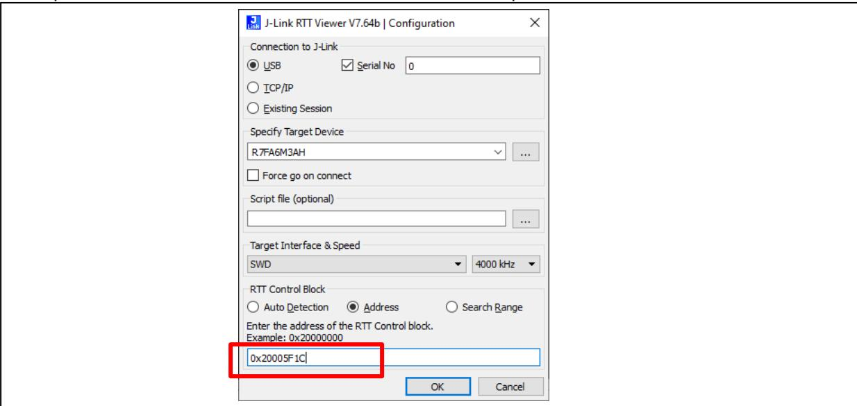
The image shows the 'J-Link RTT Viewer V7.64b | Configuration' dialog. It is set to 'USB' connection, 'R7FA6M3AH' target device, 'SWD' interface, and '4000 kHz' speed. The 'RTT Control Block' section is highlighted, showing the 'Address' radio button selected and the 'Address' input field containing the value '0x20005f1c', which is the address of the `_SEGGER_RTT` variable.
