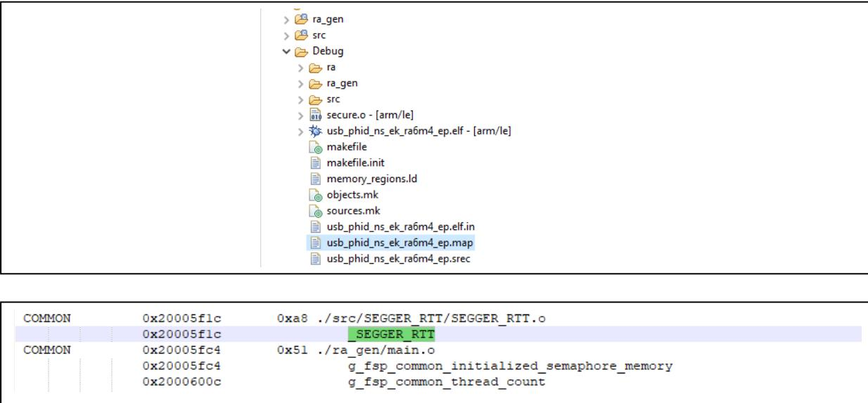
The image shows two screenshots. The top screenshot is a file explorer window showing the project structure. It includes folders for 'ra\_gen', 'src', and 'Debug', which contains files like 'ra', 'ra\_gen', 'src', 'secure.o', 'usb\_phid\_ns\_ek\_ra6m4\_ep.elf', and various build scripts. The bottom screenshot is a memory map table from a map file. It lists memory regions and their addresses, including 'SEGGER\_RTT' at address 0x20005f1c.
