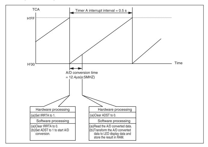
Figure 7 Description of A/D Conversion of the AN0 Pin Signal when Timer A is Used
