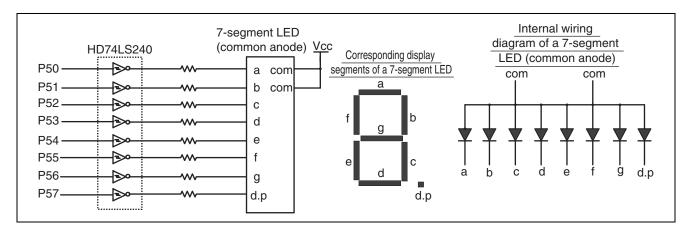
Figure 6 Connection and Internal Connections of 7-Segment LED
