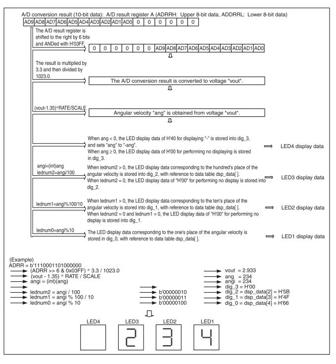
Figure 4 Display of Angular Velocity on the LEDs
