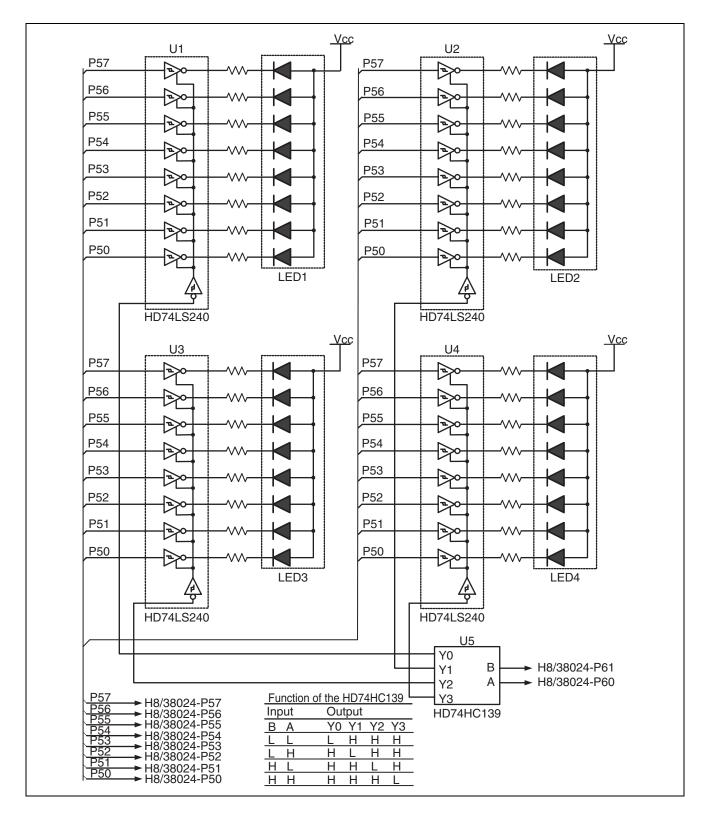
Figure 3 Control of 7-Segment LEDs
