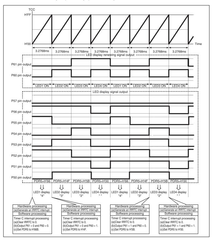
Figure 8 Description of 7-Segment LED Display Control
