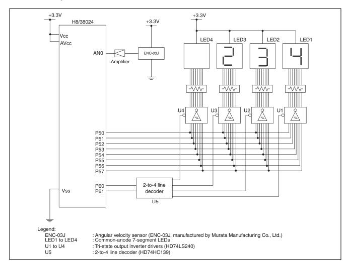
Figure 1 Hardware Configuration
