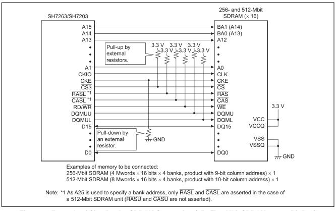
Figure 4 Example of Circuitry for SDRAM Connection (256-/512-Mbit SDRAM × 1, 16-Bit Bus)
