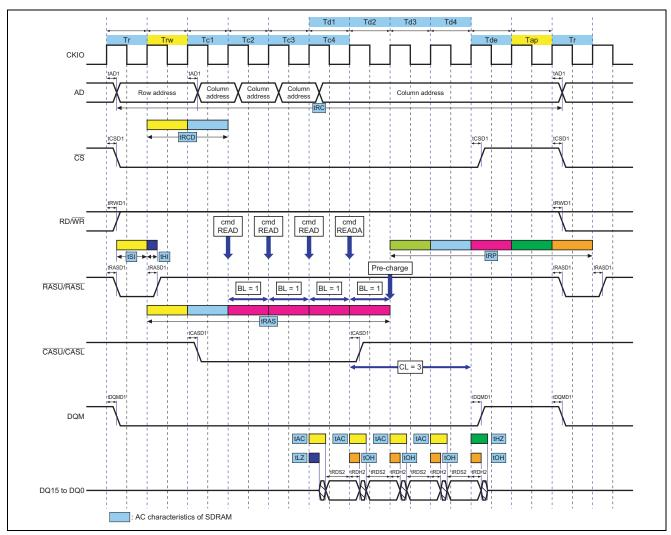
Figure 10 Timing for Burst Reading of the SDRAM (CL = 3, and WTRCD = 2, A3CL = 2 and WTRP = 1)
