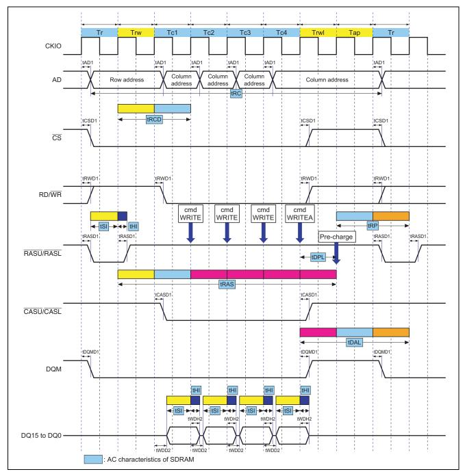
Figure 12 Timing for Burst Writing of the SDRAM (WTRCD = 2, WTRP = 1, and TRWL = 1)
