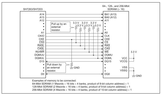
Figure 3 Example of Circuitry for SDRAM Connection (64-/128-/256-Mbit SDRAM × 1, 16-Bit Bus)
