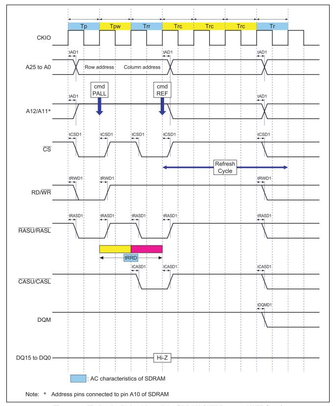
Figure 13 Timing for Refreshing of the SDRAM (WTRP = 1 and WTRC = 1)
