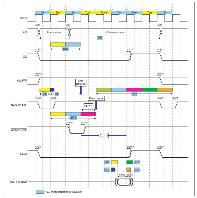
Figure 8 Timing for Single Reading of the SDRAM (CL = 3, and WTRCD = 2, A3CL = 2 and WTRP = 1)
