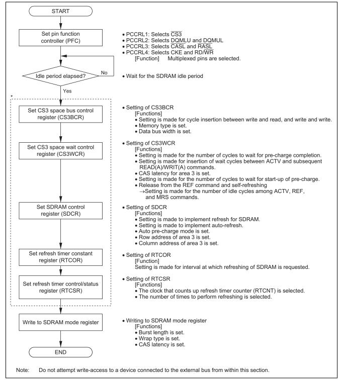
Figure 5 Example of Procedure for Initial Settings to Place SDRAM in the CS3 Space
