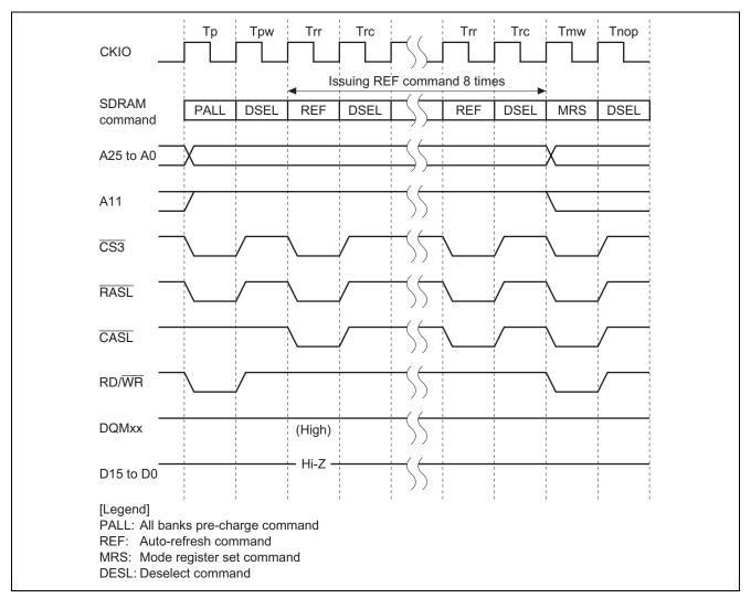
Figure 6 Example of Timing in Writing to the SDRAM Mode Register
