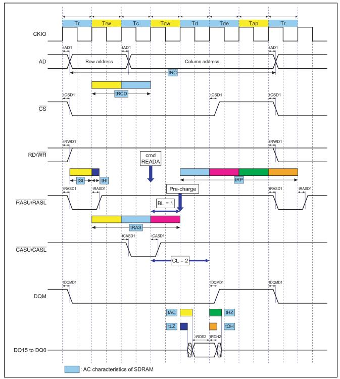
Figure 7 Timing for Single Reading of the SDRAM (CL = 2, and WTRCD = 2, A3CL = 1 and WTRP = 1)
