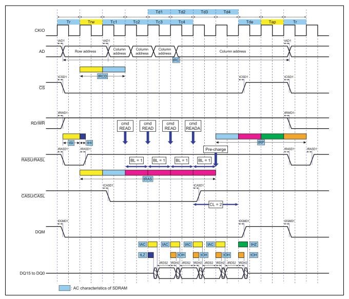
Figure 9 Timing for Burst Reading of the SDRAM (CL = 2, and WTRCD = 2, A3CL = 1 and WTRP = 1)
