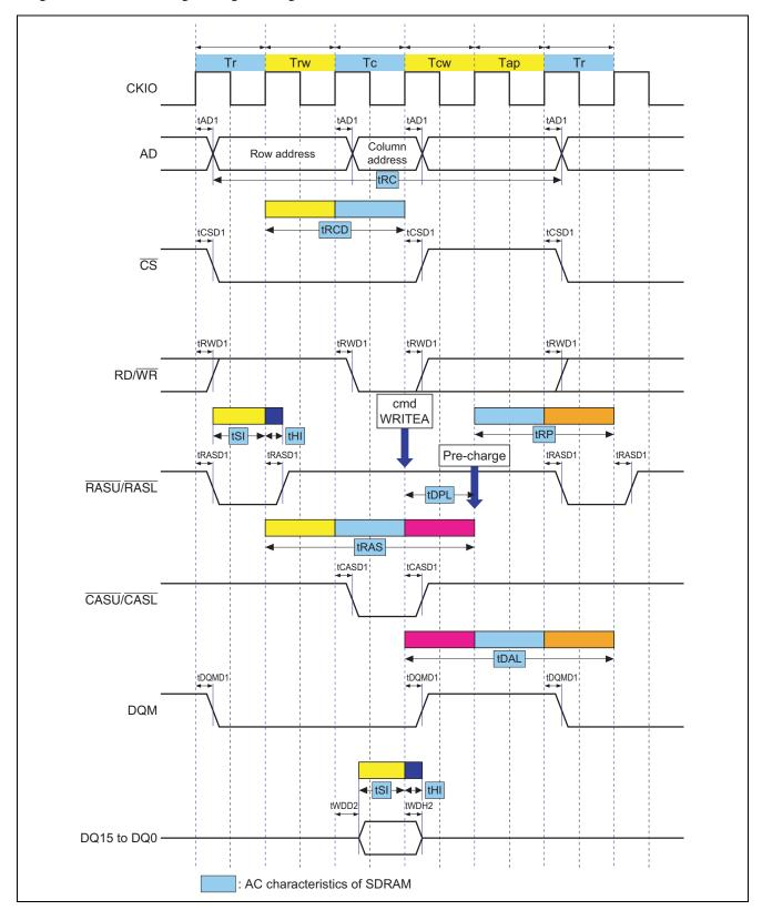
Figure 11 Timing for Single Writing of the SDRAM (WTRCD = 2, WTRP = 1, and TRWL = 1)
