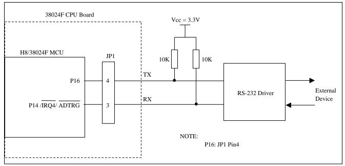
Figure 3 Micon setup with RS-232 driver
