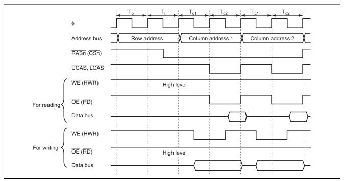
Figure 3 Burst Mode Operation Timing
