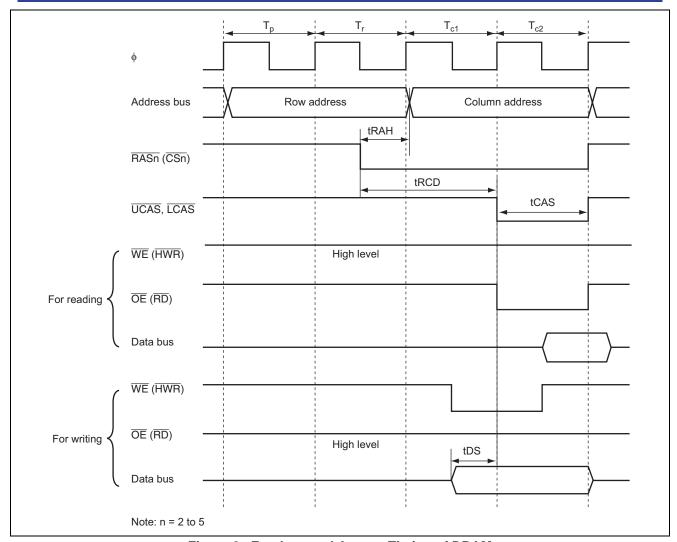
Figure 2 Fundamental Access Timing of DRAM
