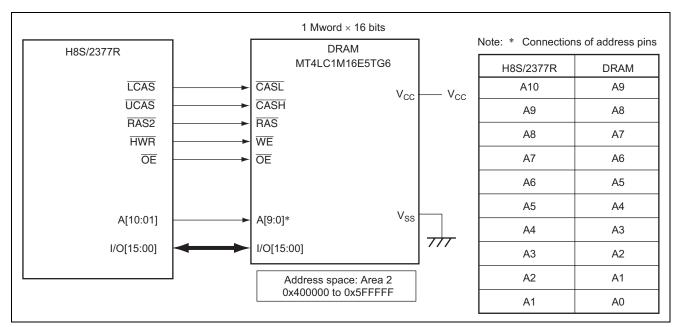
Figure 1 Connections between H8S/2377R and DRAM
