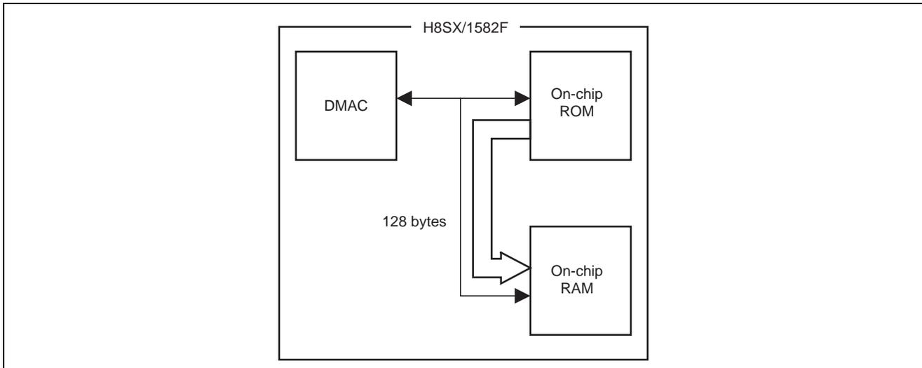
**Figure 1 Transfer by DMAC**
