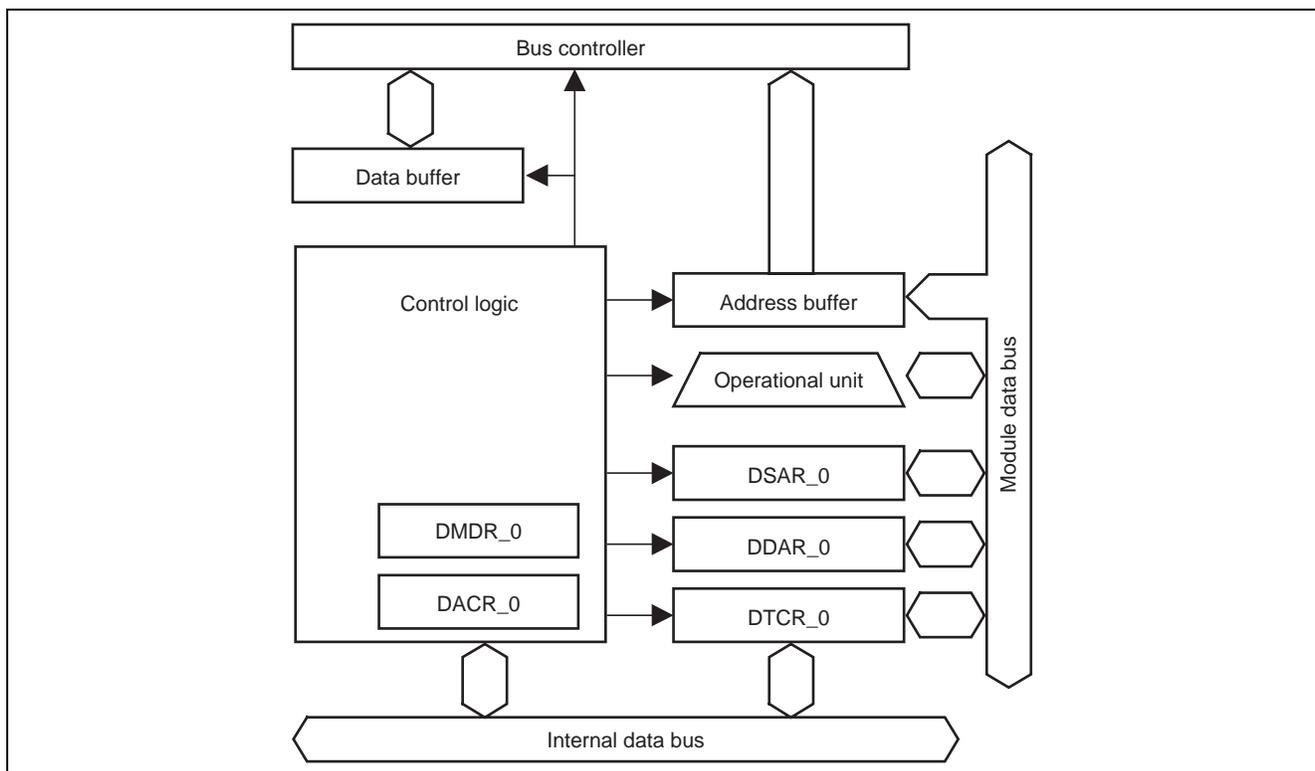
Figure 2 Block Diagram of DMAC
