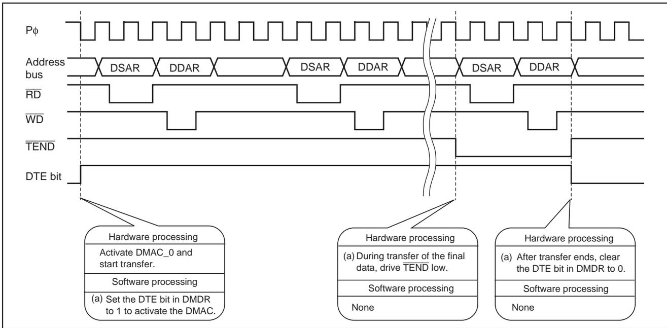
Figure 3 Example of DMA Transfer in Normal Mode
