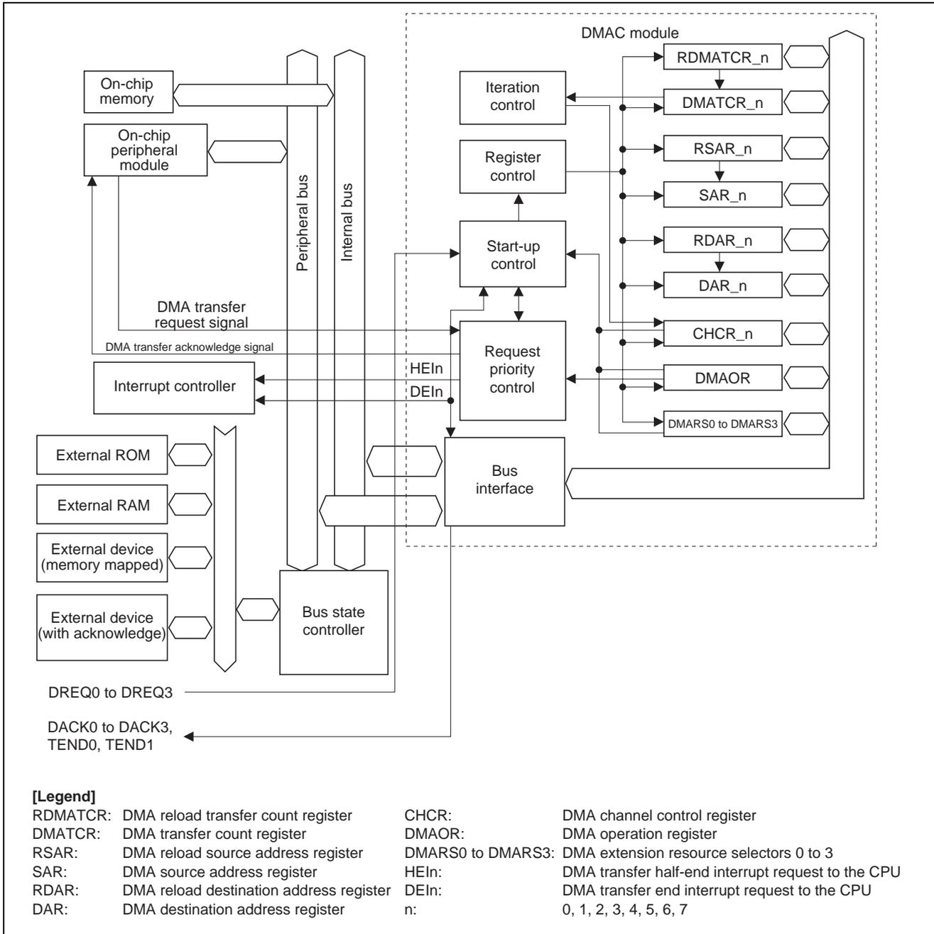
Figure 2 Block Diagram of the DMAC
