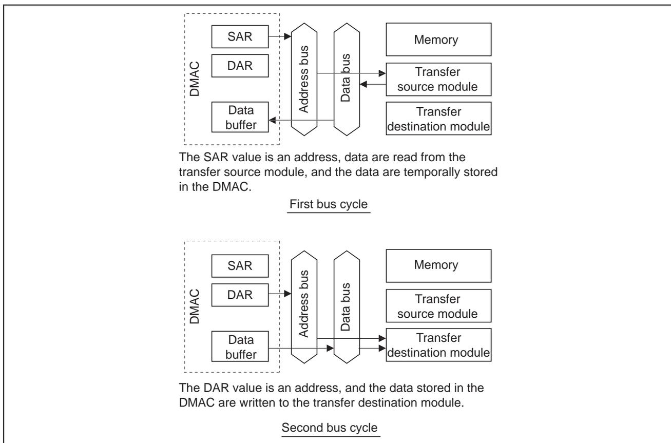
**Figure 1 Flow of Data in Dual Address Mode**
