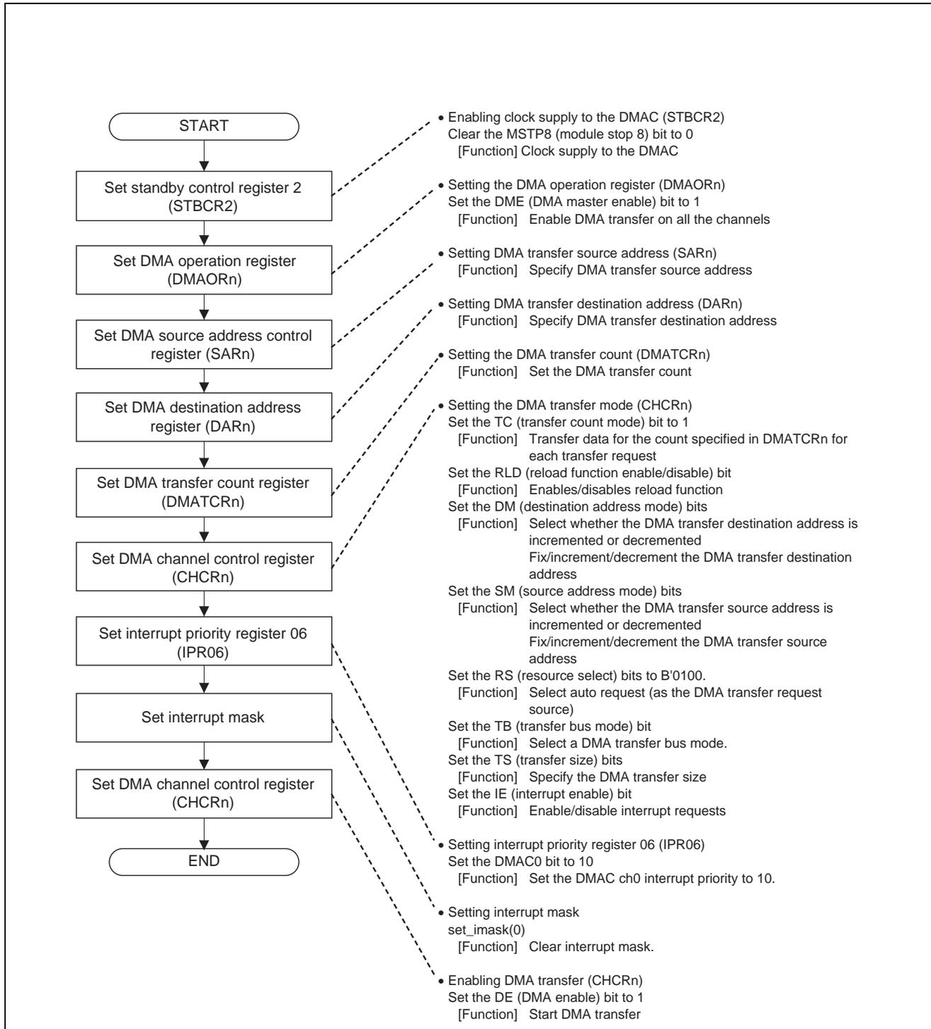
Figure 3 Flowchart of Initializing DMAC
