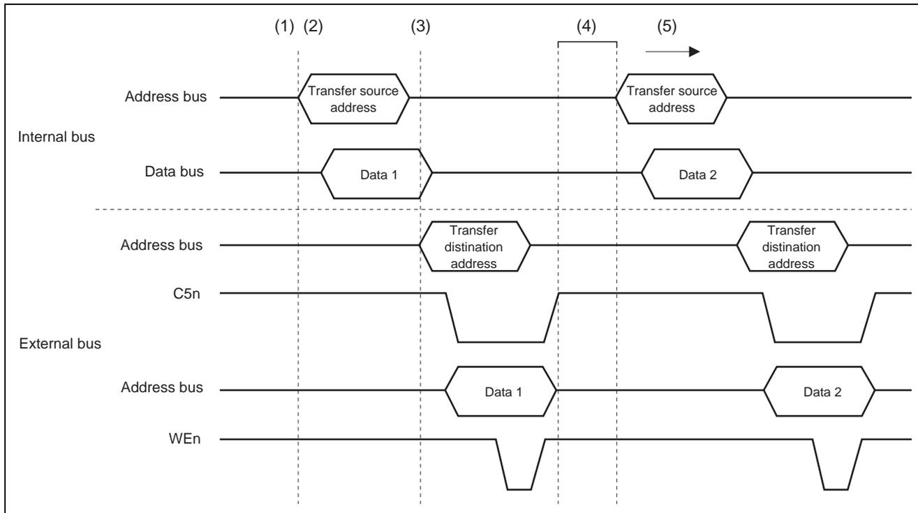
**Figure 4 Operation in Dual Address Mode**
