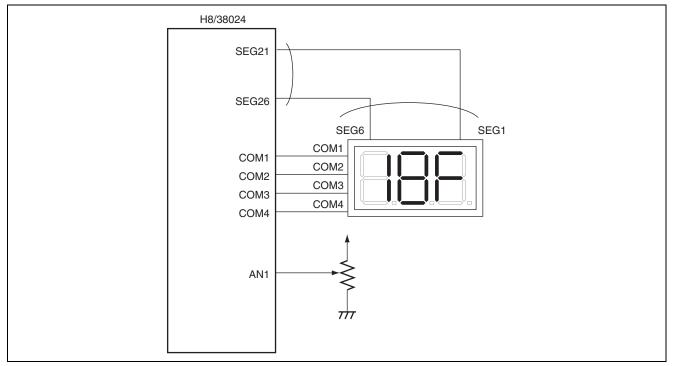
Figure 1.1 Configuration for the Sample Task
