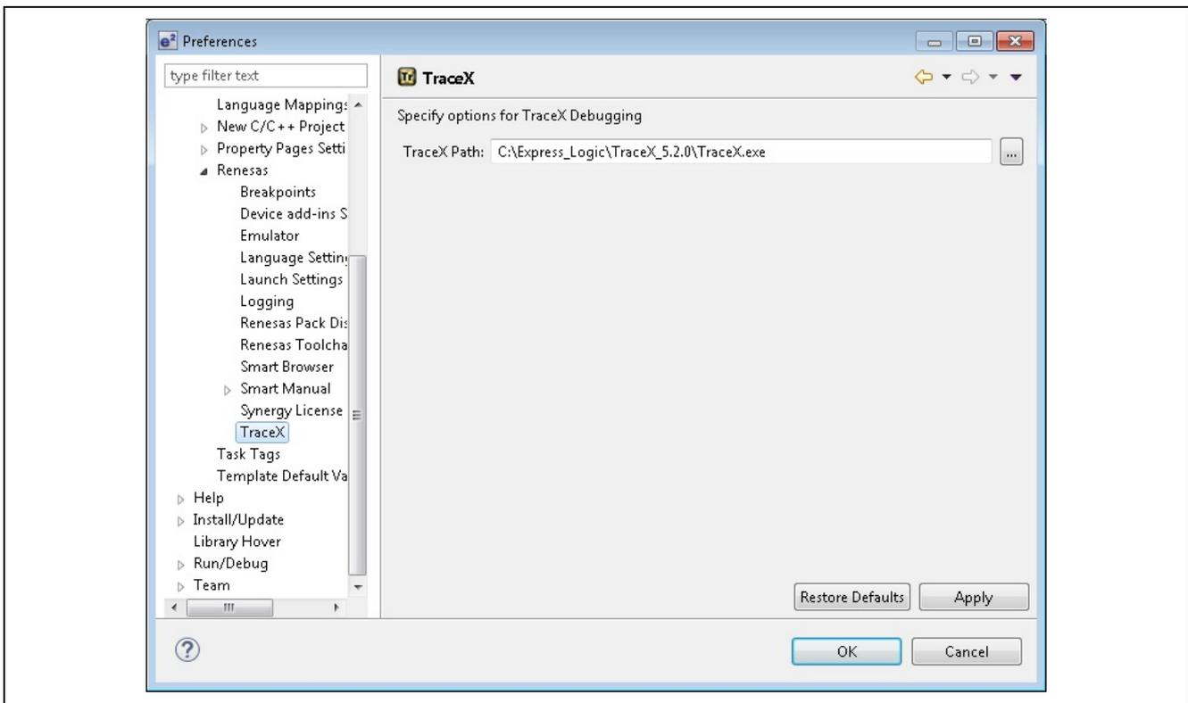
**Figure 14** Setting the TraceX path
