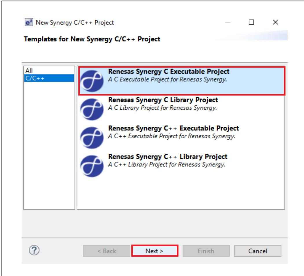
Figure 2 Selecting the Synergy C project template
