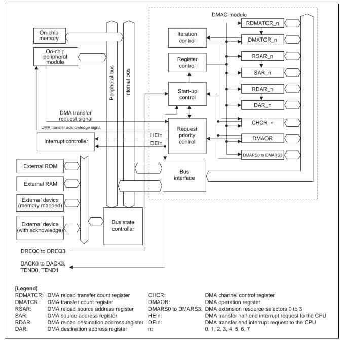
Figure 1 Block Diagram of DMAC
