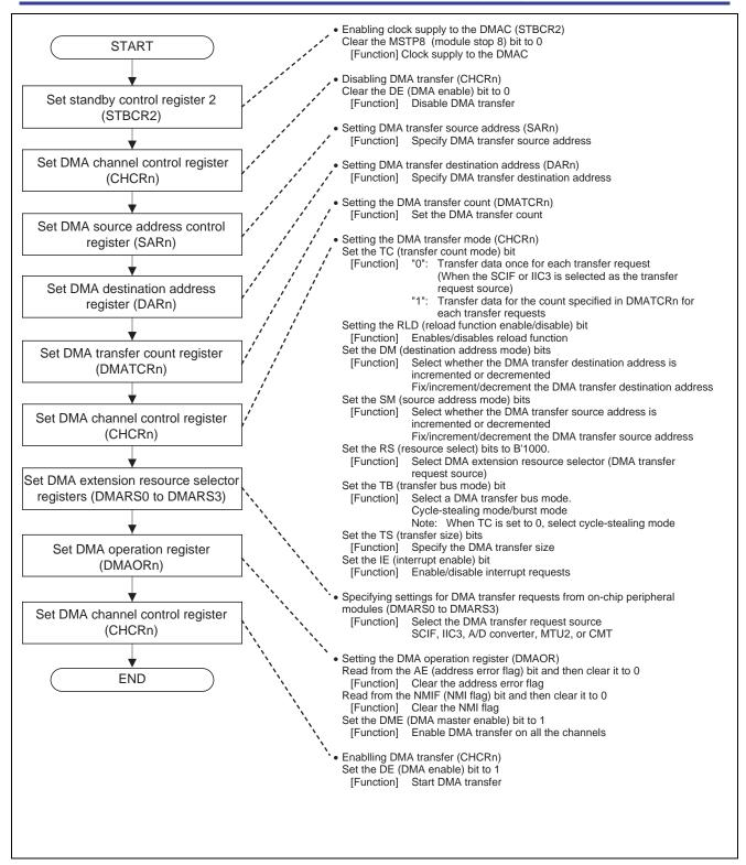
Figure 2 Flowchart of Initializing DMAC
