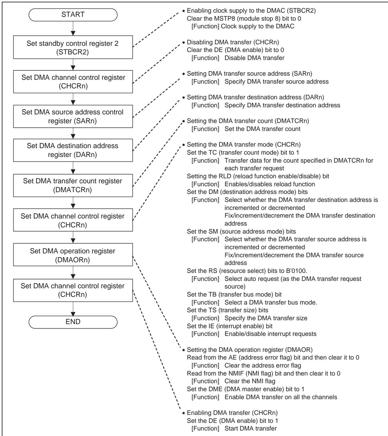
**Figure 2 Flowchart of Initializing DMAC**
