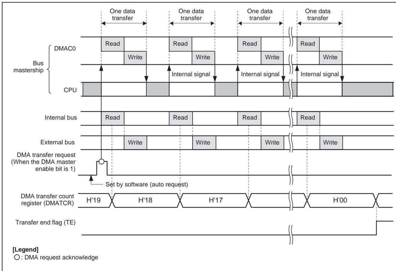
Figure 3 Operation Timing of Sample Application
