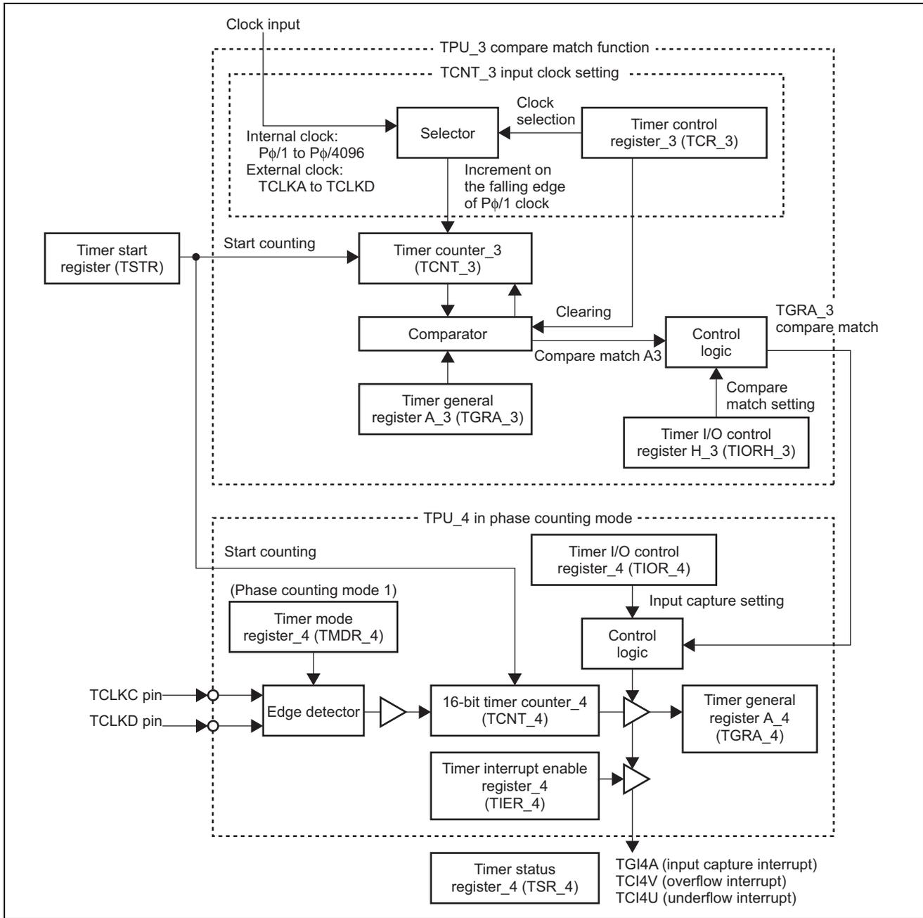
Figure 2 Block Diagram of Two-Phase Encoder Pulse Counting
