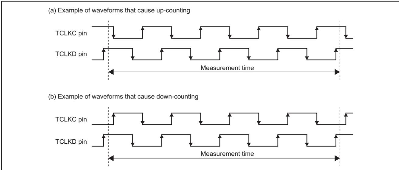
Figure 1 Counting of Two-Phase Encoder Pulse Output
