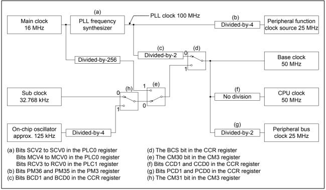
Figure 4.1 Clock Division Ratio Setting Block Diagram
