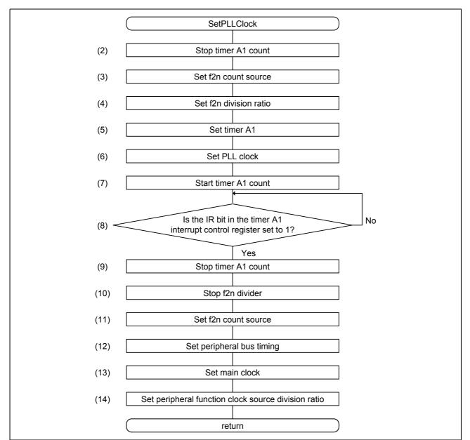
Figure 5.2 Main Clock Multiplication Mode Setting Functions
