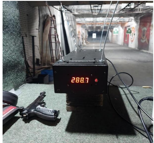
Figure 27: Cartridge Federal American Eagle CP Solid cal. 22 LR 45 gr. Beginning speed 295 m/s. Shot from Margolin pistol
