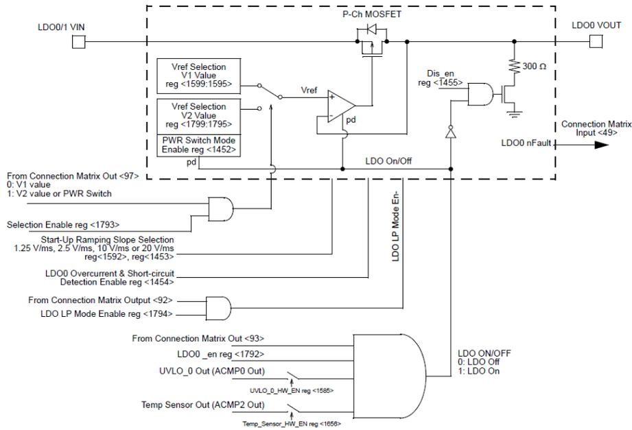
Figure 3: SLG46580 LDO0 Regulator Block Diagram
