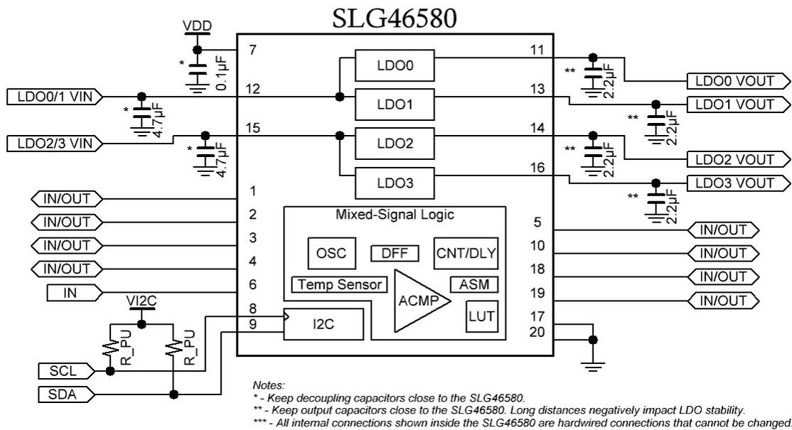
Figure 4: SLG46580 Typical Application Circuit ~ LDO Configuration
