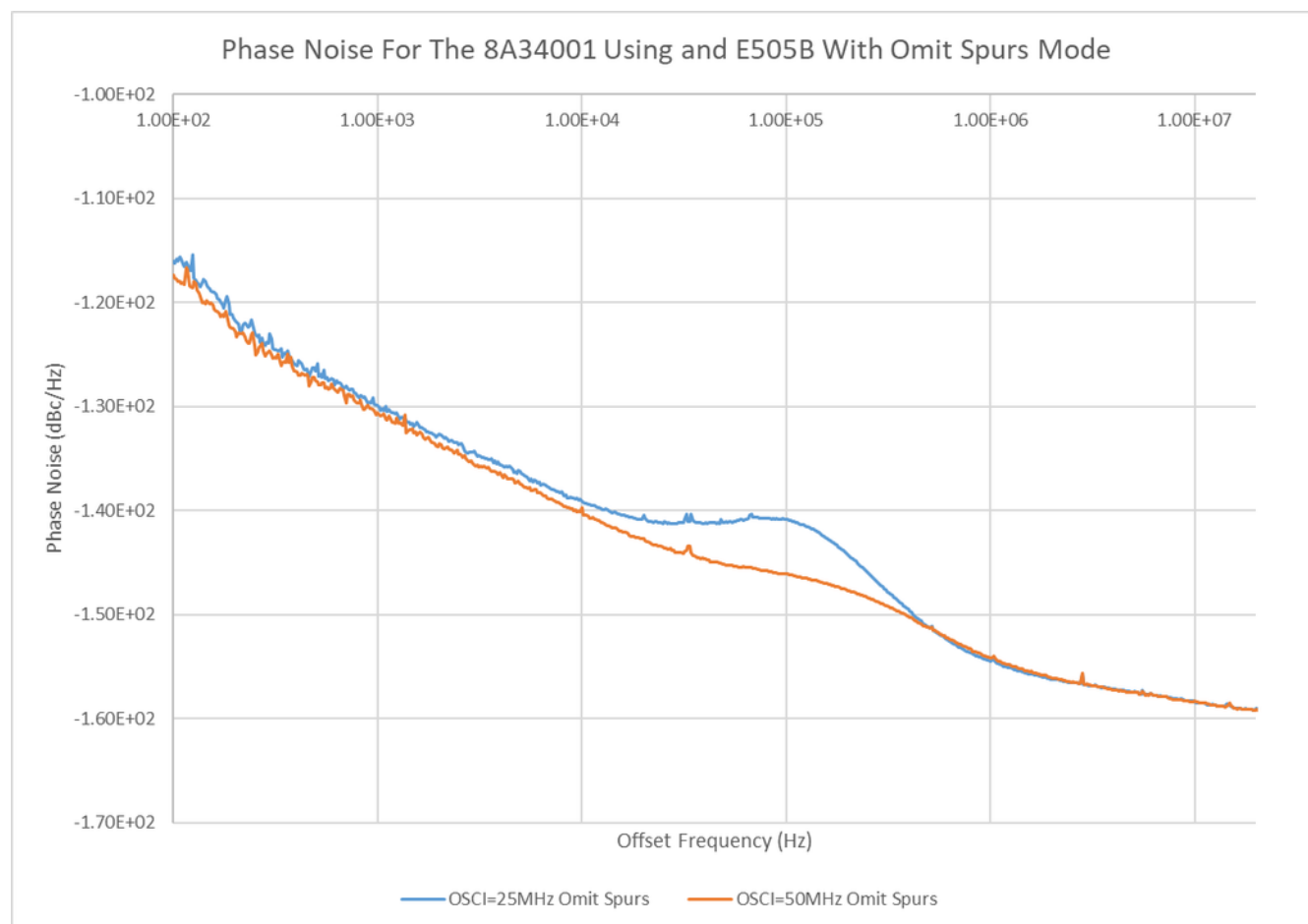
Figure 2. Phase Noise Plots of a Clock Synthesizer using a 25MHz Crystal Compared to a 50MHz Crystal
