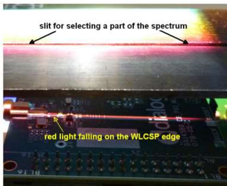
Figure 6: Dark red light falling on the WLCSP
