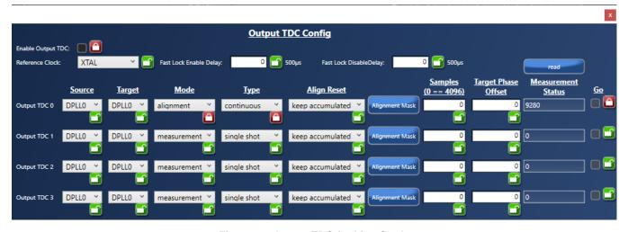
Figure 27. Output TDC for Line Card
