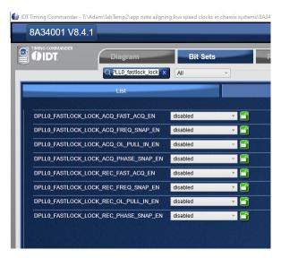
Figure 9. DPLL Channel 0 Fast Lock Settings for Master
