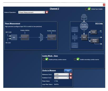
Figure 13. Phase Measurement (Channel 2) for Master
