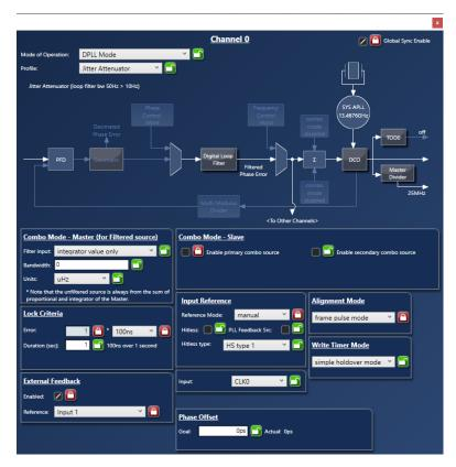
Figure 21. DPLL Channel 0 Configuration for Line Card
