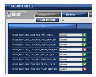
Figure 12. DPLL Channel 1 Fast Lock Settings for Master
