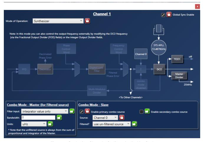
Figure 26. Synthesizer Channel 1 Configuration for Line Card
