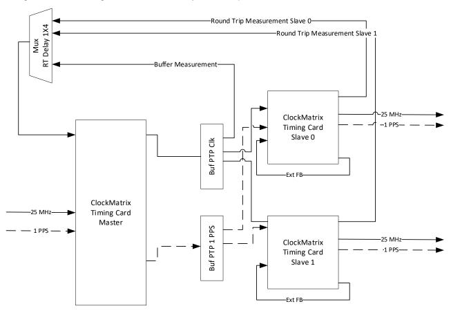
Figure 1. Example System using Paired Clocks
