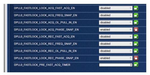
Figure 23. DPLL Channel 0 Fast Lock Register Configuration for Line Card
