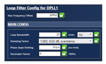
Figure 11. DPLL Channel 1 Loop Filter for Master
