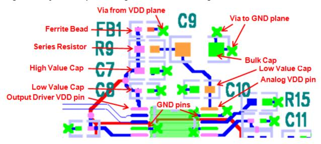
The capacitors most effective at preventing EMI in this layout example are C8 and C10.
