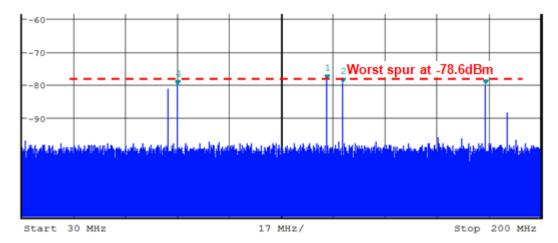
81MHz = -80.2dBm 78MHz = -81dBm 130MHz = -78.6dBm 135MHz = -79.6dBm
