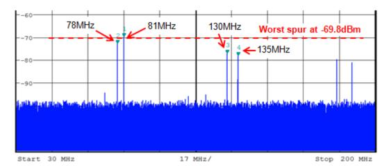
81MHz = -69.8dBm 78MHz = -73.1dBm 130MHz = -77.3dBm 135MHz = -78.2dBm
